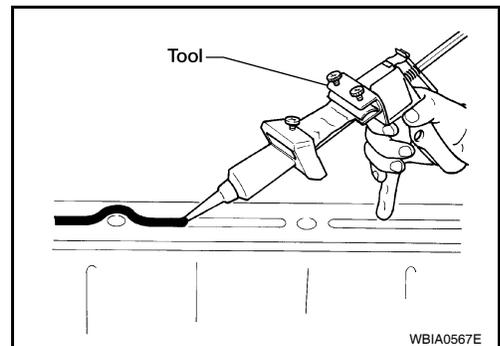
4. Apply liquid gasket without breaks to the specified location with the specified dimensions.
