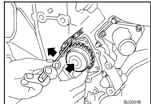
4. Remove dust and foreign material completely from backside of chain tensioner and from installation area of rear timing chain case.
