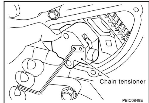
12. Remove the three water pump bolts. Make a gap between water pump gear and timing chain, by turning crankshaft pulley counterclockwise until timing chain loosens on water pump sprocket.
