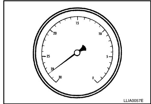
9. When the vacuum gauge has reached the specified amount, disconnect the air hose and wait 20 seconds to see if the system loses any vacuum. If the vacuum level drops, perform any necessary repairs to the system and repeat steps 6 - 8 to bring the vacuum to the specified amount. Recheck for any leaks.
