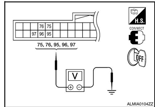
Is the measurement normal when any of the switches is turned ON?
