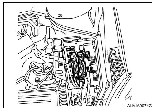
4. While depressing the tabs (A) remove the IPDM E/R (1) from the vehicle.
