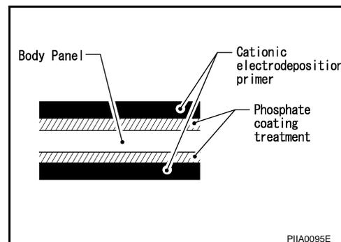
Nissan Genuine Service Parts are also treated in the same manner. Therefore, it is recommended that GENUINE NISSAN PARTS or equivalent be used for panel replacement to maintain anti-corrosive performance built into the vehicle at the factory.
