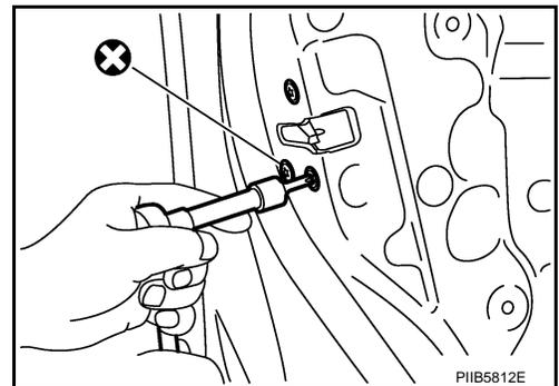
8. Remove the TORX bolt (T30), and remove the outside handle bracket.
