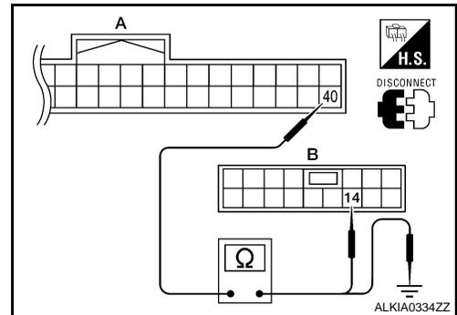
3. Check continuity between BCM connector M18 (A) terminal 40 and ground.
