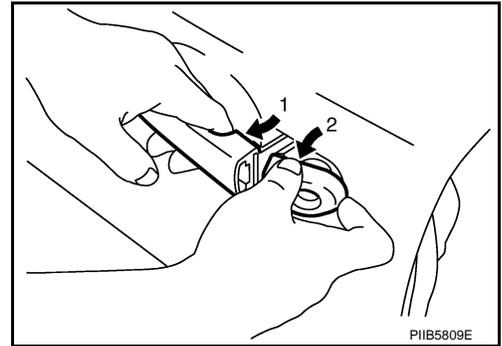
7. Disconnect front door request switch harness connector (with Intelligent Key system).
