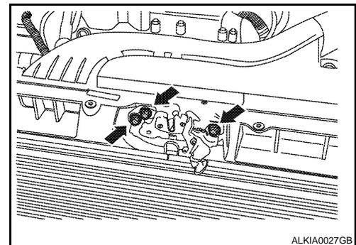
4. Disconnect the hood lock cable from the hood lock, and unclip it from the hoodledge.
