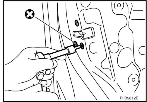
11. Remove the TORX bolt (T30) of the outside handle bracket.
