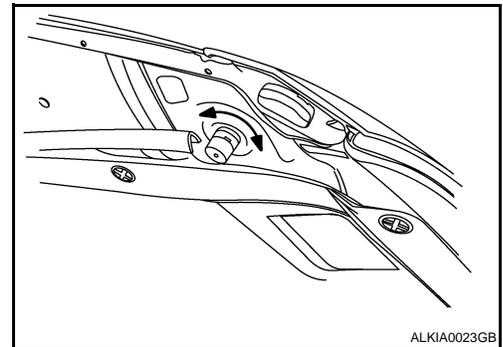
5. Install and align the hood lock center with the center of the hood striker. Engage the lock with the striker and check for looseness.
