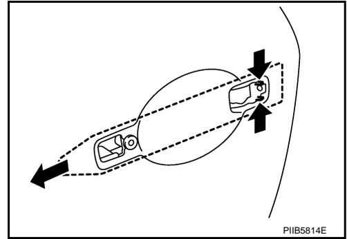
10. Disconnect the door lock actuator connector and remove the door lock assembly.
