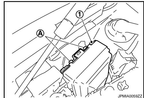
4. Remove the IPDM E/R cover A while pressing the pawl (A) at the lower end of the IPDM E/R cover A (1).
