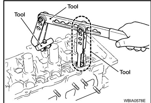
4. Remove valve oil seal using Tool.
