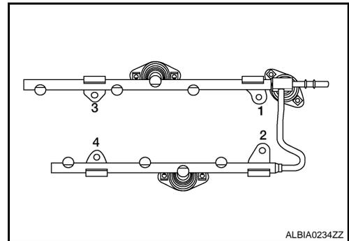
3. Install the intake manifold collector bolts in the numerical order as shown.
