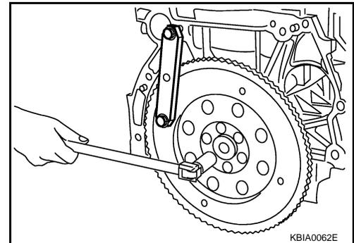
8. Remove pilot converter using Tool (CVT models).
