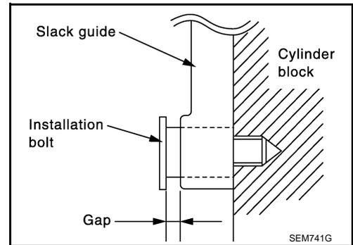
13. Install the timing chain tensioner for the slack guide.
