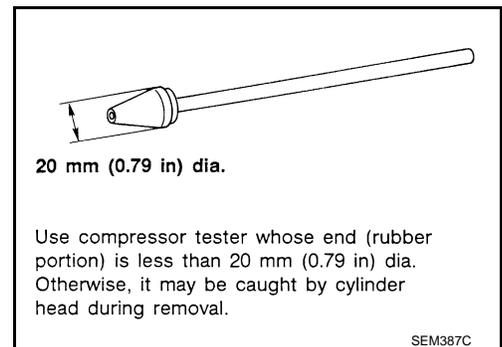
7. With the accelerator pedal fully depressed, turn the ignition switch to the "START" position to crank over the engine. When the gauge pointer stabilizes, read the compression pressure and engine rpm. Perform these steps to check each cylinder.
