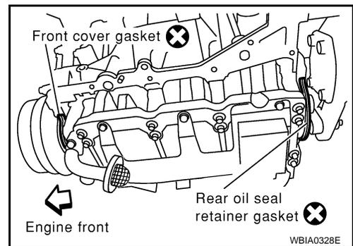
4. Apply a bead of sealant to the cylinder block mating surface of the upper oil pan to a limited portion as shown.
