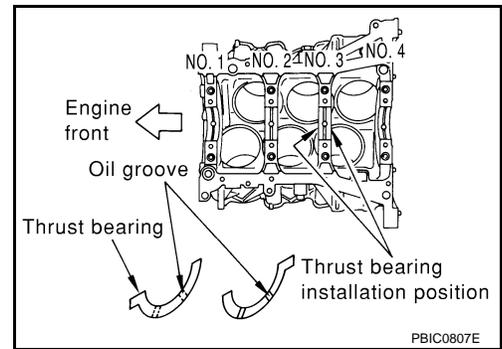
5. Set the upper main bearings in their proper positions on the cylinder block.
