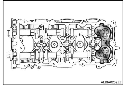
4. Remove the intake and exhaust camshaft brackets and the camshafts.
