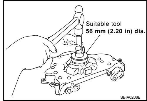
7. Install front cover with the following procedure:
