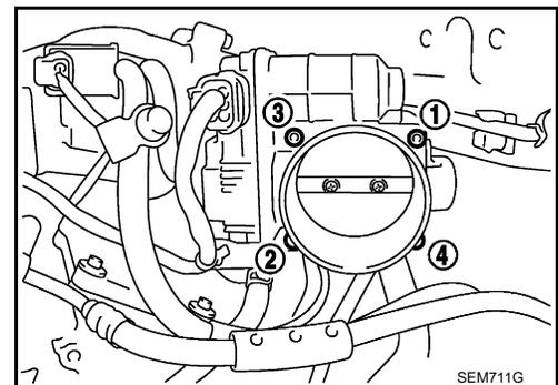
11. If necessary, remove power valve bolts in the order as shown and remove the power valve.
