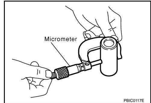
Connecting Rod Bushing Oil Clearance (Small End)
