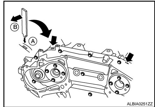
33. Remove the front oil seal from the front timing chain case using a suitable tool.
