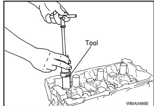
5. Turn crankshaft until the cylinder requiring new oil seals is at TDC. This will prevent valve from dropping into cylinder.
