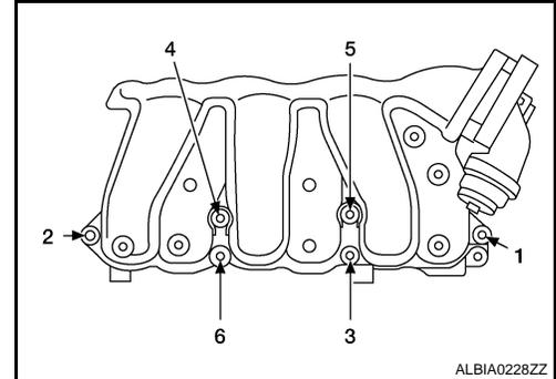
10. If necessary, remove the electric throttle control actuator bolts in the order as shown and remove the electric throttle control actuator.
