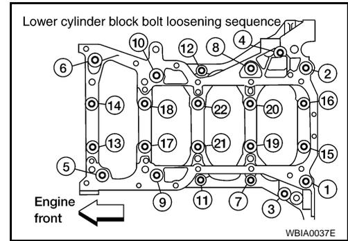
14. Remove the lower cylinder block.
