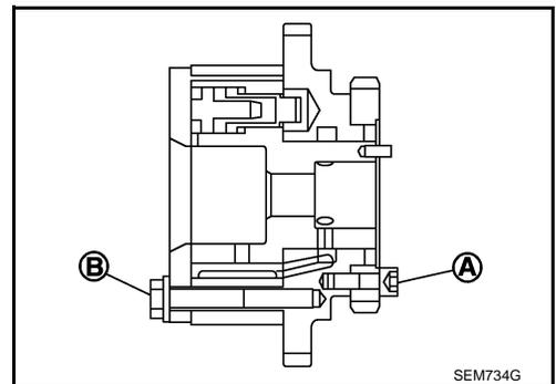
19. Remove the chain tension guide.
