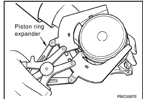
14. Remove the piston from the connecting rod as follows.
