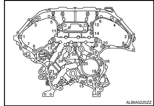
21. Remove O-rings to timing chain case and cylinder block.
