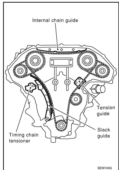
14. Remove the timing chain tensioner and slack side chain guide.
