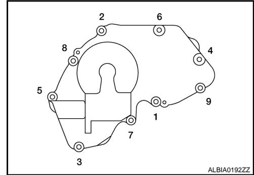
Remove the IVT (intake valve timing) control cover using Tool.
