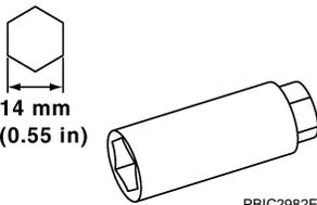
PBIC2982E | Removing and installing spark plug                                                                           | P           |
