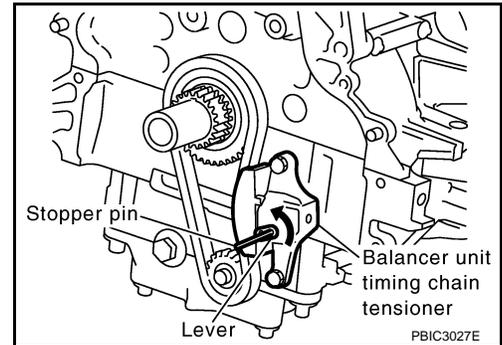
22. Loosen bolts in order as shown, and remove balancer unit.
