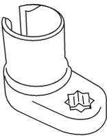
LEM054    | Loosening or tightening air fuel ratio (A/F) sensor 1                                  | D<br>E<br>F         |
