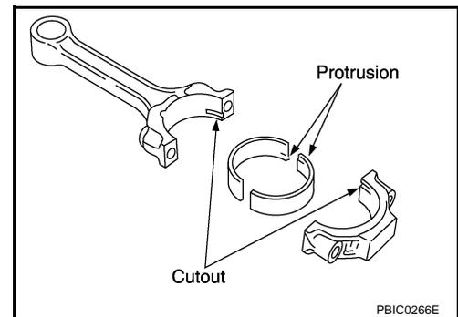
13. Install the piston and connecting rod assembly into the corresponding cylinder.
