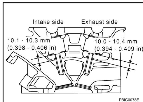
6. Apply finish to valve guide using suitable reamer.
