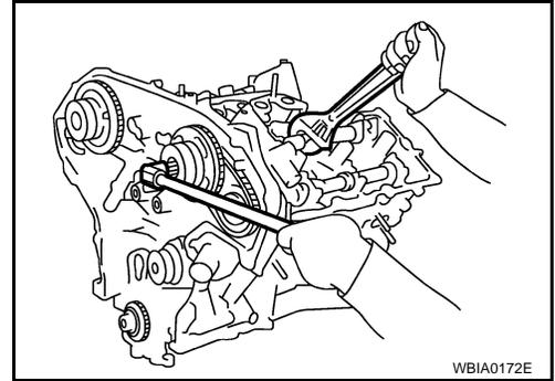
18. Remove the secondary timing chains with camshaft sprockets.
