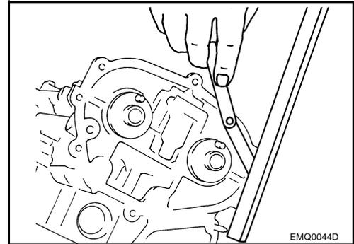
9. Install the IVT control solenoid valves with new gaskets.
