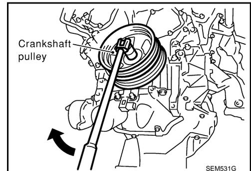
13. Rotate crankshaft pulley in normal direction (clockwise when viewed from front) to confirm it turns smoothly.
