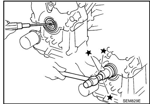
34. Use a scraper to remove all of the old Silicone RTV Sealant from the front timing chain case and opposite mating surfaces.
