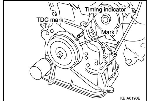
5. At this time, check that the both intake and exhaust cam lobes of No. 1 cylinder face outside.
