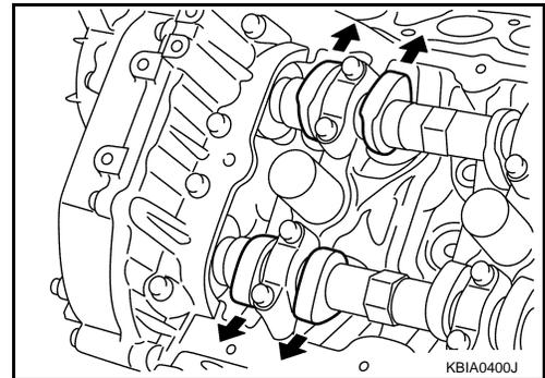
6. By referring to the figure (locations indicated with black arrow), measure valve clearances with a feeler gauge at locations marked X as shown in the table below.
