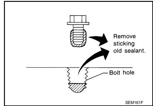
2. Before installing the front cam bracket, remove the old Silicone RTV Sealant from the mating surface using a scraper.
