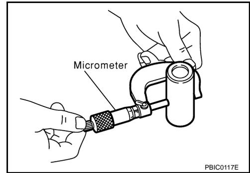
Connecting Rod Bushing Oil Clearance (Small End)
