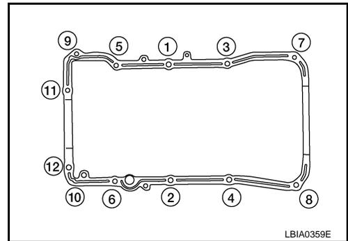
7. Install the four upper oil pan to transaxle bolts.
