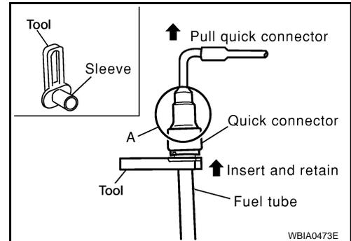
8. When removing fuel hose quick connector at vehicle piping side, perform as follows.
