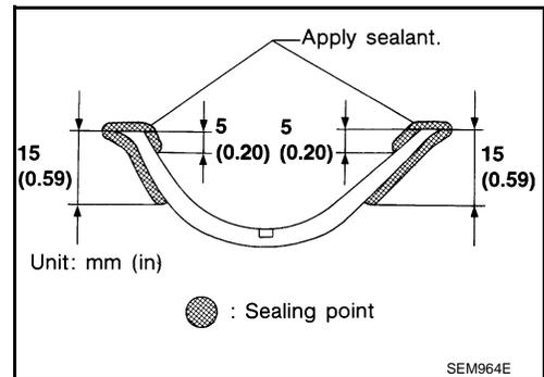
3. Install the front cover gasket and rear oil seal retainer gasket as shown.
