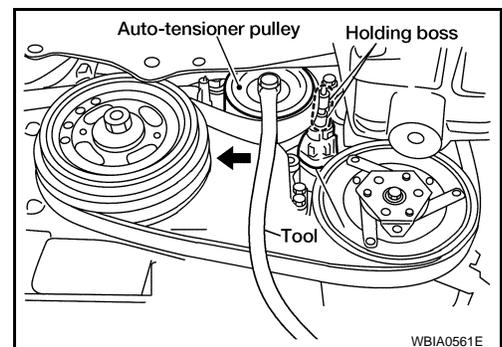
2. Insert a rod approximately 6 mm (0.24 in) in diameter through the rear of tensioner into retaining boss to lock tensioner pulley.
