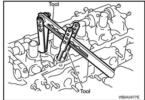
5. Remove valve oil seal using Tool.
