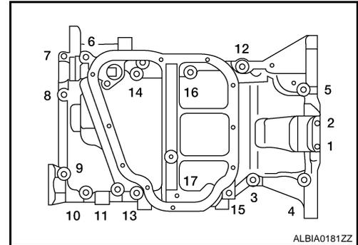
11. Remove upper oil pan using Tool.
