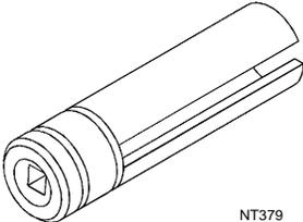
NT379 | Loosening or tightening heated oxygen sensor<br><b>For 22 mm (0.87 in) hexagon nut</b> | A<br><b>EM</b><br>C |
