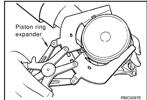
12. Remove the piston from the connecting rod as follows.
