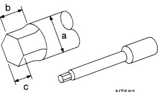
NT583<br>Loosening and tightening cylinder head bolt<br><b>a: 13 (0.51) dia.</b><br><b>b: 12 (0.47)</b><br><b>c: 10 (0.39)</b><br>Unit: mm (in) |
