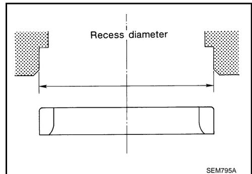
**Be sure to ream in circles concentric to the valve guide center.**
