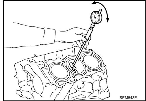
If it exceeds the limit, rebore all cylinders. Replace cylinder block if necessary.
