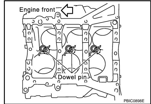
4. Install the main bearings and the thrust bearings.
