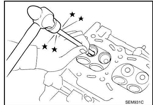
3. Ream cylinder head valve guide hole using suitable reamer.
