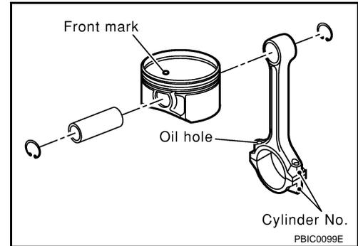
10. Using a piston ring expander, install the piston rings. Assemble the components in their original positions.
