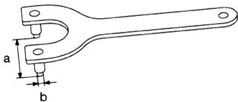
NT628         | Crankshaft pulley removing and installing<br><b>a: 68 mm (2.68 in) dia.</b><br><b>b: 8 mm (0.31 in) dia.</b> | J<br>K<br>L |
