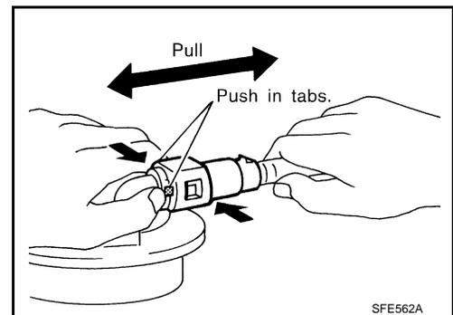
9. Disconnect throttle control actuator coolant hoses.
