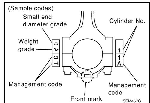
**Factory installed parts grading:**
