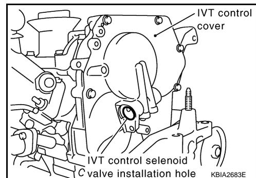
5. Clean oil groove between oil strainer and IVT control solenoid valve if engine oil does not come out from IVT control cover oil hole. Refer to [LU-6](#), "[Lubrication Circuit](#)".
