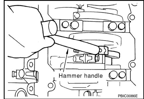
12. Remove the connecting rod bearings.
