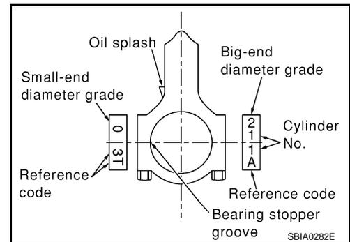
2. Apply pin diameter grade stamped on crankshaft front side to the column in the "Connecting Rod Bearing Selection Table".
