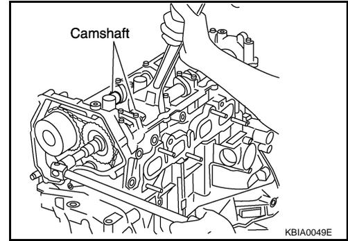
18. Remove the chain slack guide, tension guide, timing chain, and oil pump drive spacer.
