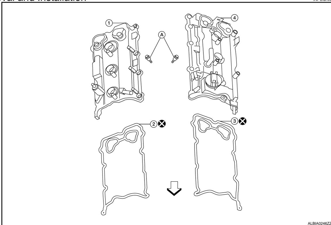
1. Rocker cover (RH)                      2. Rocker cover gasket (RH)                      3. Rocker cover gasket (LH)
