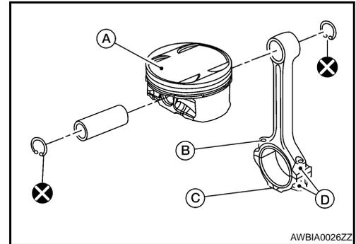
b. Install the piston to the connecting rod.
