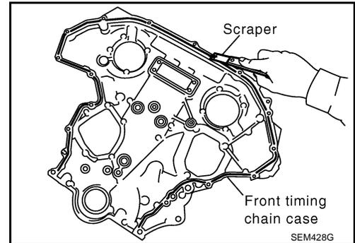
23. Remove all old Silicone RTV Sealant from all the bolt holes and bolts.
