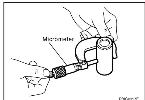
Piston to Piston Pin Clearance
