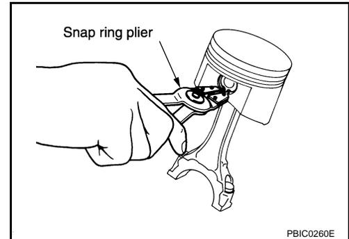
b. Heat the piston to 60° - 70°C (140° - 158°F) with a heat gun, or equivalent.
