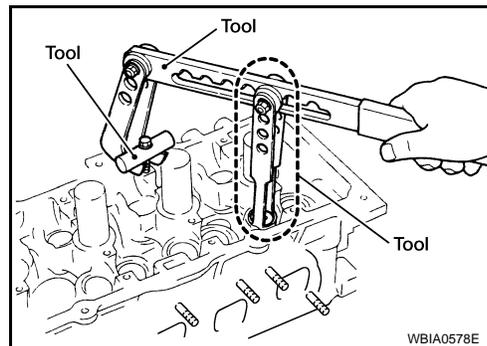
4. Remove valve spring retainer, valve spring and valve spring seat.
