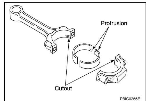
12. Install the piston and connecting rod assembly to the crankshaft. Assemble the components in their original positions.
