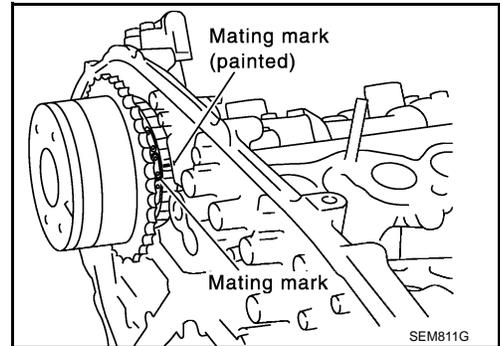
7. After confirming the mating marks are aligned, tighten the camshaft sprocket bolts.
