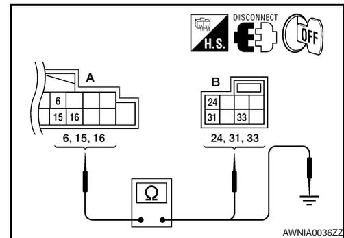
4. Check continuity between audio unit connector M43 (A) and ground.
