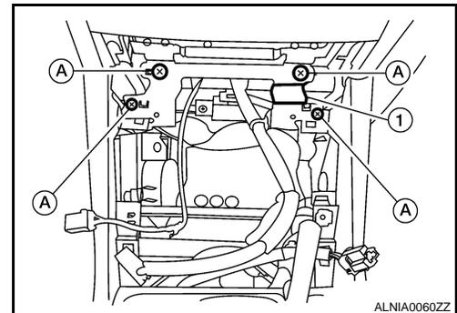
5. Pull out the navigation audio unit assembly, disconnect the navigation audio unit assembly connectors.
