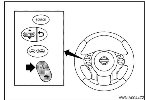
4. While the prompt is playing, press and hold the steering wheel audio control switch END button until you hear the “Diagnostics mode” prompt. The Bluetooth system will sound a 5 second beep.
