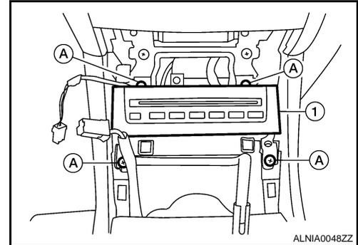
6. Remove the CD changer bracket screws (A).
