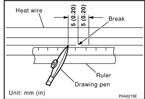
4. After repair has been completed, check repaired wire for continuity. This check should be conducted 10 minutes after silver composition is deposited. Do not touch repaired area while test is being conducted.
