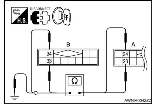
4. Check continuity between satellite radio tuner (factory installed) and ground.
