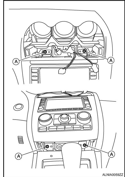
4. Remove the navigation audio unit bracket screws (A) and remove the navigation audio unit bracket (1).
