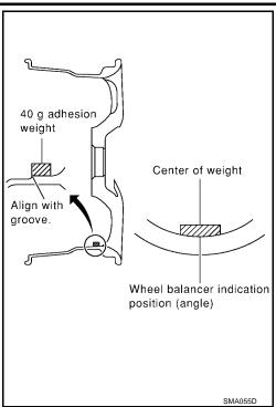
c. If calculated balance weight value exceeds 50 g (1.76 oz.), install two balance weight sheets in line with each other as shown.
