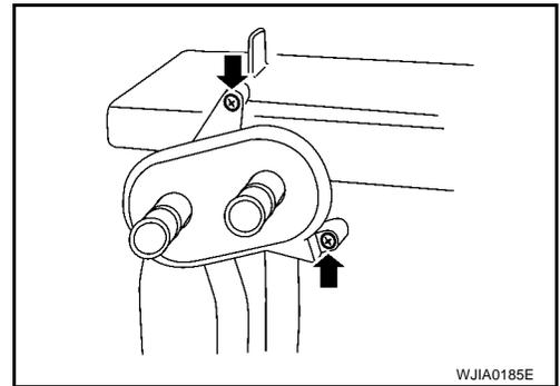
3. Remove the heater core cover screws and then remove the heater core cover.
