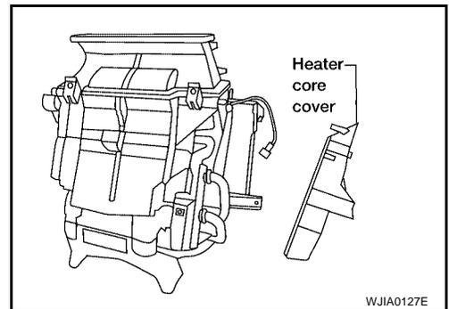
4. Remove the heater core.
