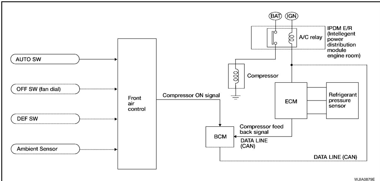
The ECM controls compressor operation using input signals from the throttle position sensor and front air control.
