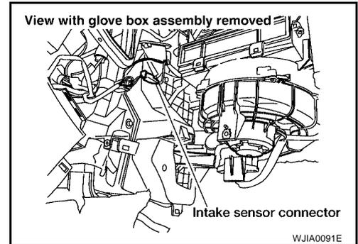
If NG, replace intake sensor. Refer to [ATC-90, "INTAKE SENSOR"](#).
