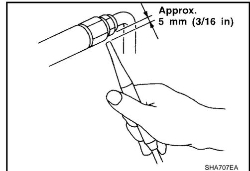
2. When testing, circle each fitting completely with the leak detector probe.
