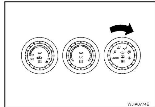
2. Confirm that discharge air comes out according to the air distribution table below.
