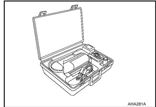
1. Position the leak detector probe approximately 5 mm (3/16 in) away from the point to be checked.
