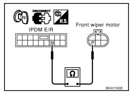
Check continuity between front wiper motor harness connector terminal E and body ground.
