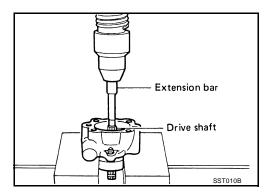
Remove oil seal. Be careful not to damage front housing.
