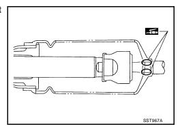
5. Install the boot clamps and crimp securely.
