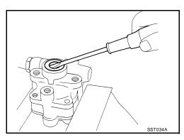
3. Remove connector and flow control valve with spring. Be careful not to drop flow control valve.
