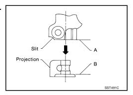
After installation, turn steering wheel to make sure it moves smoothly. Ensure the number of turns are the same from the straight-forward position to left and right locks. Be sure that the steering wheel is in a neutral position when driving straight ahead.
