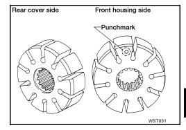
When assembling vanes to rotor, rounded surfaces of vanes must face cam ring side.
