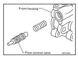
4. Inspect all of the power steering oil pump components, and repair or replace as necessary. Refer to PS-24, "Inspection After Disassembly".
