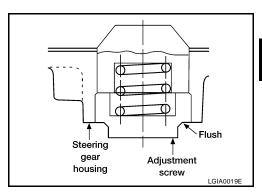
2. Loosen adjusting screw in  $40^{\circ}$  -  $60^{\circ}$  increments until rack sliding force is within specification.
