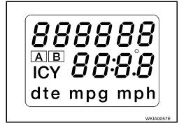
7. Push the odo/trip meter switch. Each meter/gauge should indicate as shown in the figure while pushing odo/trip meter switch. (at this time, the low-fuel warning lamp goes off).
