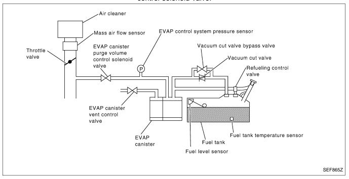
Malfunction is detected when EVAP control system has a leak, EVAP control system does not operate properly.
