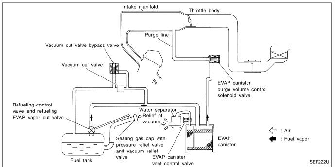
The evaporative emission system is used to reduce hydrocarbons emitted into the atmosphere from the fuel system. This reduction of hydrocarbons is accomplished by activated charcoals in the EVAP canister.
