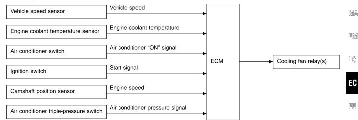
The ECM controls the cooling fan corresponding to the vehicle speed, engine coolant temperature, air conditioner system pressure and air conditioner ON signal. The control system has 3-step control [HIGH/LOW/OFF].
