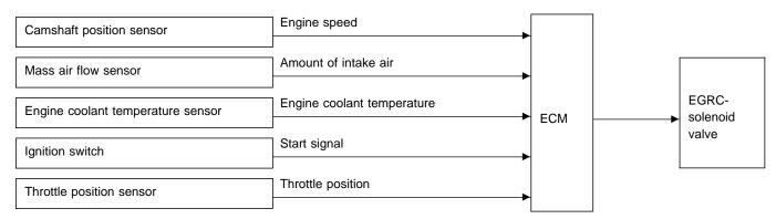
This system cuts and controls vacuum applied to the EGR valve to suit engine operating conditions. This cut-and-control operation is accomplished through the ECM and the EGRC-solenoid valve. When the ECM detects any of the following conditions, the ECM cuts the current for the solenoid valve. This causes the port vacuum to be discharged into the atmosphere. The EGR valve remains closed.
