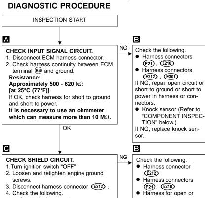
Continuity between harness connector (E212) terminal (2) and ground Continuity should exist.
