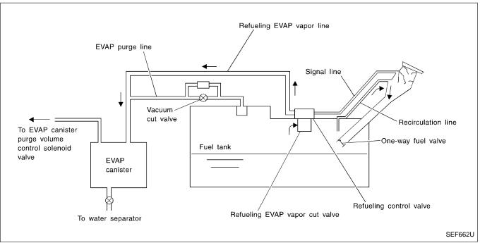
From the beginning of refueling, the fuel tank pressure goes up. When the pressure reaches the setting value of the refueling control valve (RCV) opening pressure, the RCV is opened. After RCV opens, the air and vapor inside the fuel tank go through refueling EVAP vapor cut valve, RCV and refueling vapor line to the EVAP canister. The vapor is absorbed by the EVAP canister and the air is released to the atmosphere.
