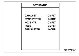
A sample of CONSULT-II display for SRT code is shown at left. "INCMP" means the self-diagnosis is incomplete and SRT is not set. "CMPLT" means the self-diagnosis is complete and SRT is set.
