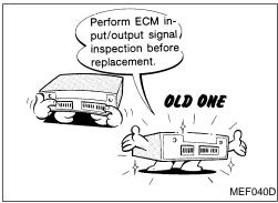
Before replacing ECM, perform Terminals and Reference Value inspection and make sure ECM functions properly. Refer to EC-98.
