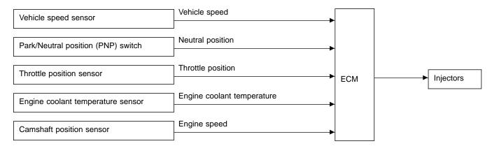
If the engine speed is above 4,000 rpm with no load, (for example, in neutral and engine speed over 4,000 rpm) fuel will be cut off after some time. The exact time when the fuel is cut off varies based on engine speed.
