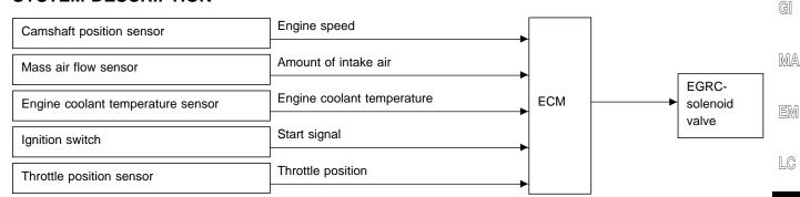
This system cuts and controls vacuum applied to the EGR valve to suit engine operating conditions. This cut-and-control operation is accomplished through the ECM and the EGRC-solenoid valve. When the ECM detects any of the following conditions, it cuts the current for the solenoid valve. This causes the port vacuum to be discharged into the atmosphere. The EGR valve remains closed.
