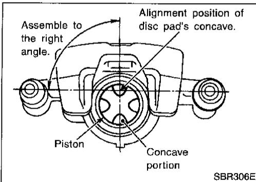
10. Adjust the piston to the right angle as shown in the figure.
