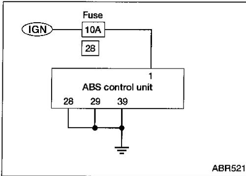
1. Disconnect control unit connectors. Check terminals for damage or loose connections. Then reconnect connectors.
