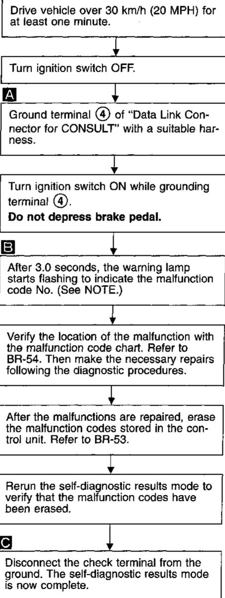
**NOTE:** The indication terminates after five minutes. However, when the ignition switch is turned from OFF to ON, the indication starts flashing again.
