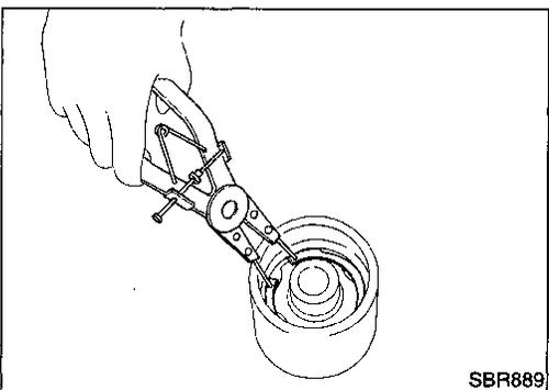
2. Remove snap ring from piston with suitable pliers and remove adjusting nut.
