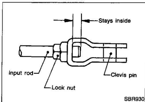
If necessary, adjust brake pedal free height.
