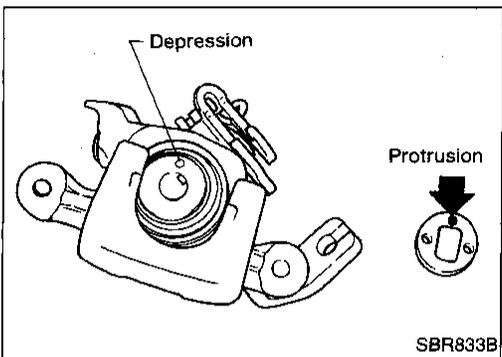
3. Match protrusion on key plate with depression in cylinder.
