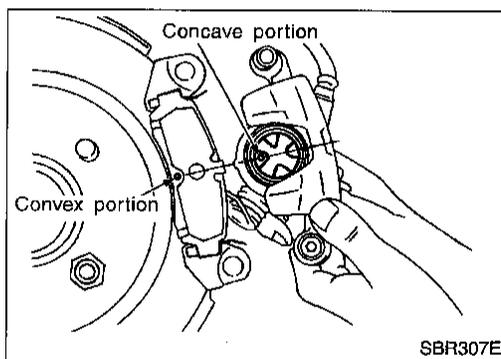
8. As shown in the figure, align the piston's concave to the pad's convex, then install the cylinder body to the torque member.
