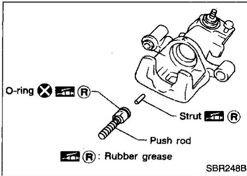
2. Generously apply rubber grease to strut and push rod to make insertion easy.
