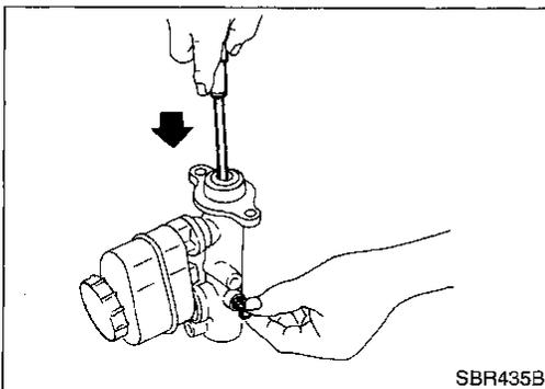
5. Install valve stopper while piston is pushed into cylinder. (Models with ABS only)
