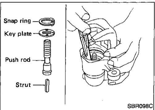
4. Install snap ring with a suitable tool.
