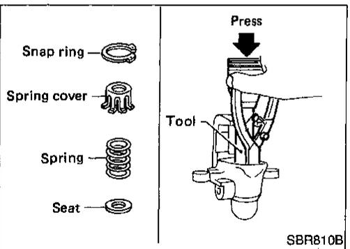
5. Install seat, spring, spring cover and snap ring while depressing with a suitable tool.
