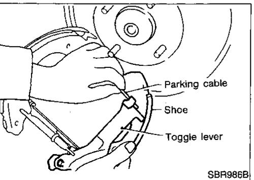
6. Connect parking brake cable to toggle lever.
