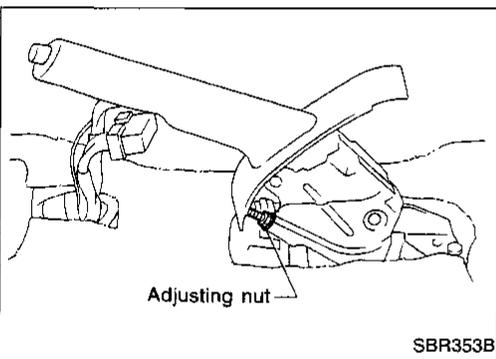
2. Pull control lever 4 - 5 notches. Then adjust control lever by turning adjusting nut.
