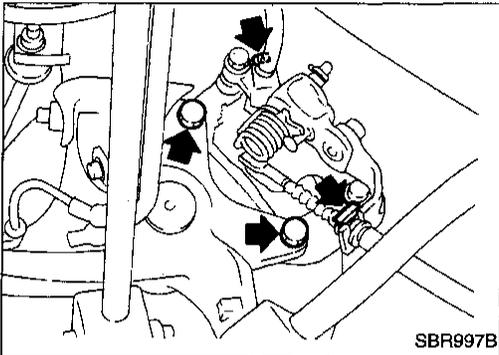
1. Remove brake cable mounting bracket bolt and lock spring.
