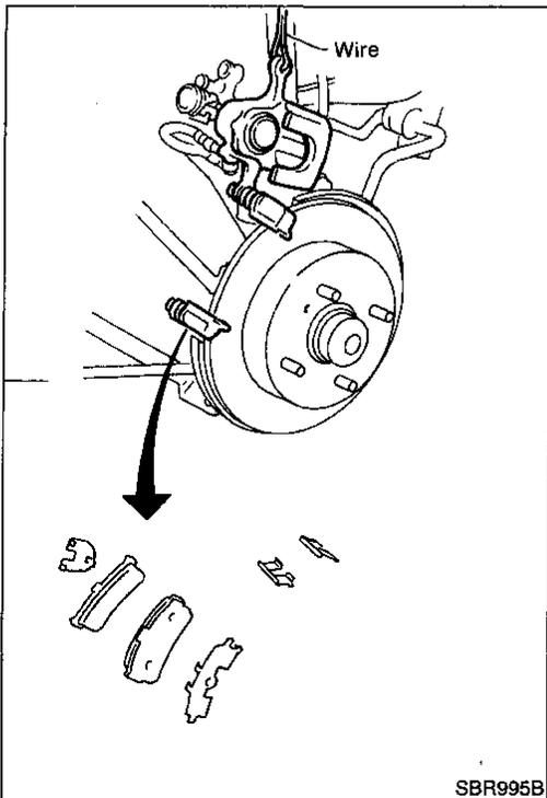
5. Open cylinder body upward. Then remove pad retainers, and inner and outer shims.
