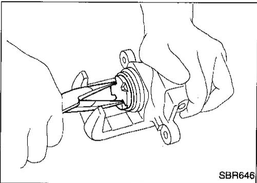
8. Insert piston seal into groove on cylinder body.
