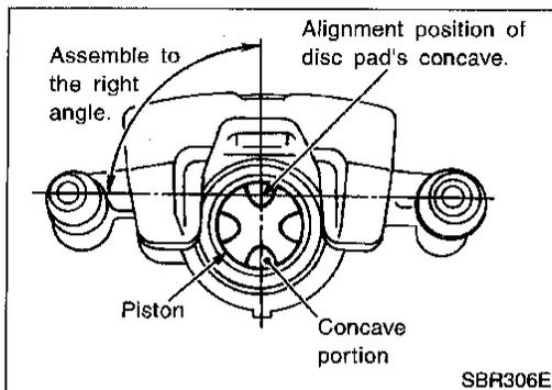
7. Adjust the piston to the right angle as shown in the figure.
