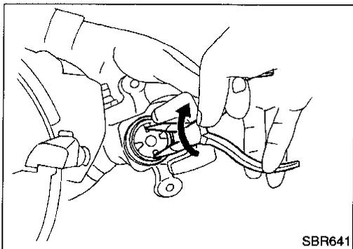
6. When installing new pads, push piston into cylinder body by turning piston clockwise.
