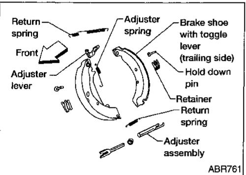
5. Install adjuster and adjuster lever; then install upper return spring and adjuster spring.
