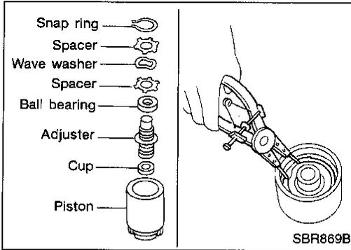
7. Install cup, adjuster, bearing, spacers, washer and snap ring with a suitable tool.
