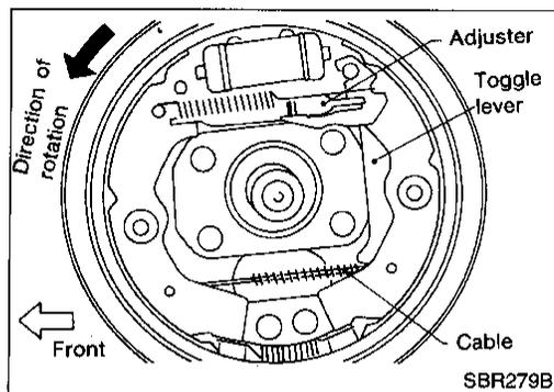
9. Secure shoe installation with shoe hold-down pins and retainers.
