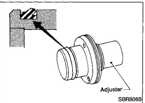
6. Install adjuster in the specified direction.
