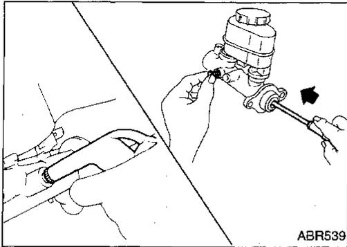
2. Remove valve stopper while piston is pushed into cylinder (Models with ABS only).
