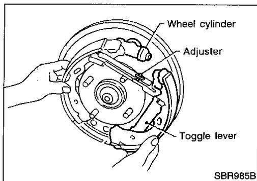
7. Install shoes on wheel cylinder one at a time.
