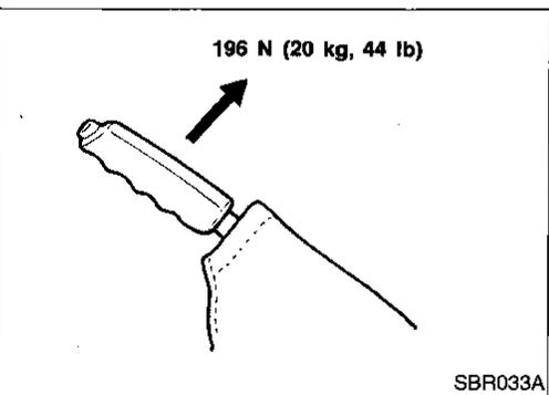
3. Pull control lever with specified amount of force. Check lever stroke and ensure smooth operation.
