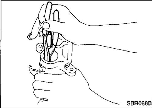
3. Disassemble cylinder body.
