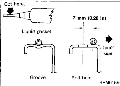
11. Apply a continuous bead of liquid gasket to mating surface of steel oil pan.
