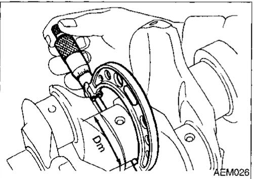
**When grinding crankshaft journal, confirm that "L" dimension in fillet roll is more than the specified limit.**
