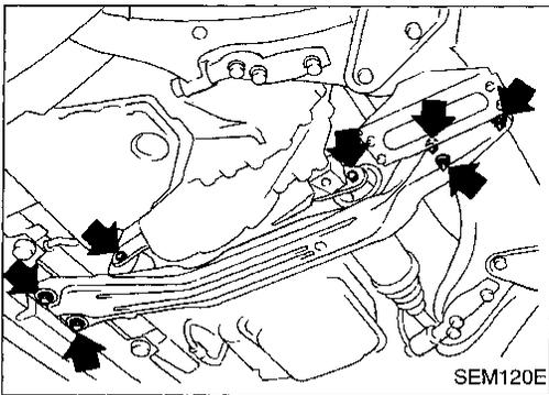
13. Remove engine with transaxle as shown.
