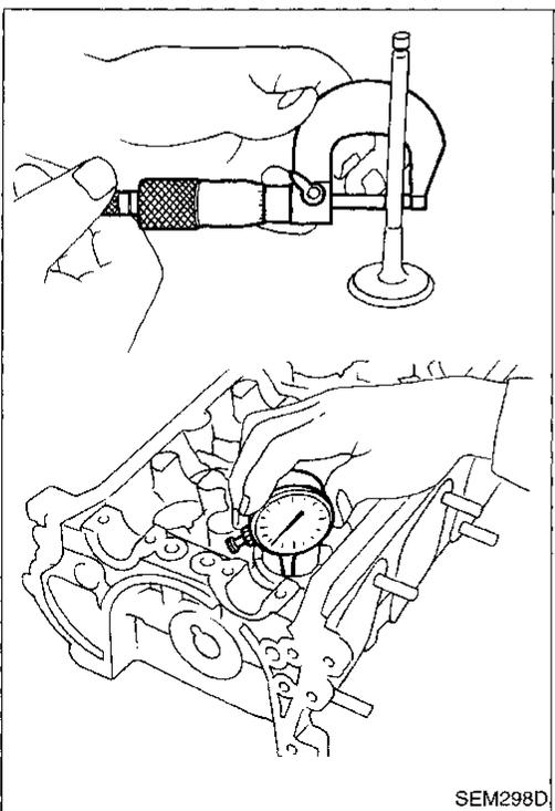
2. If it exceeds the limit, check valve to valve guide clearance.
