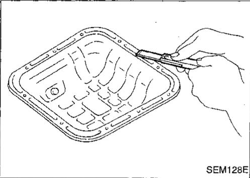
10. Use a scraper to remove old liquid gasket from mating surface of steel oil pan.
