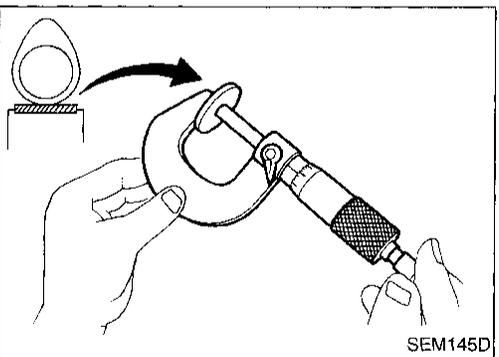
7. Determine replacement adjusting shim size as follows:
