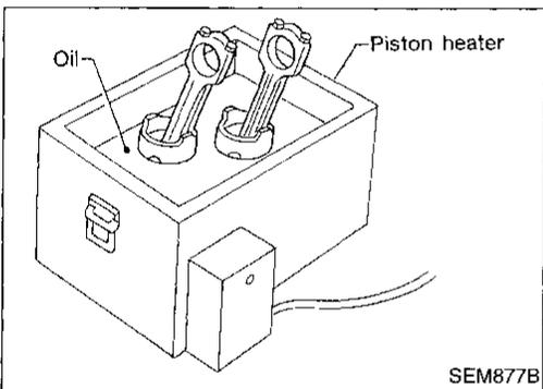
3. Remove pistons with connecting rods.
