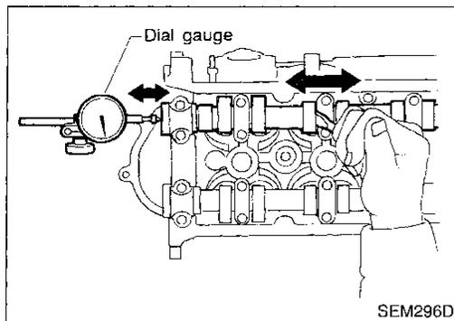
1. Install camshaft in cylinder head. Refer to EM-24.
