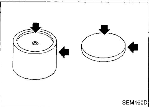
2. Check diameter of valve lifter and valve lifter guide bore.
