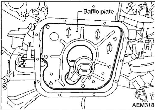
5. Remove baffle plate.
