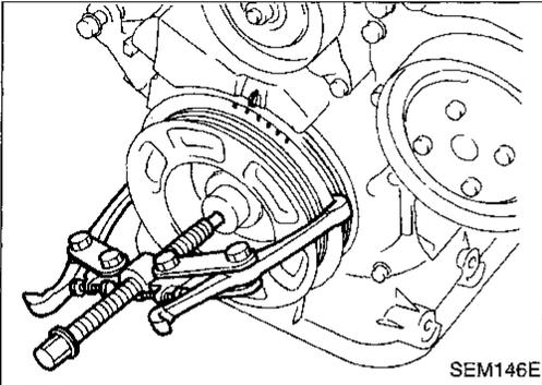
3. Remove crankshaft pulley.
