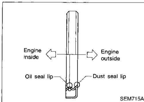
3. Apply engine oil to new oil seal and install it using a suitable tool.
