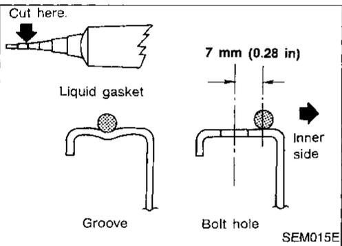
2. Apply a continuous bead of liquid gasket to mating surface of aluminum oil pan.
