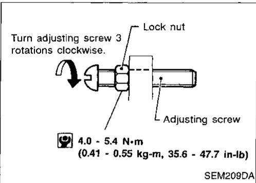
9. Turn adjusting screw 3 rotations clockwise.
