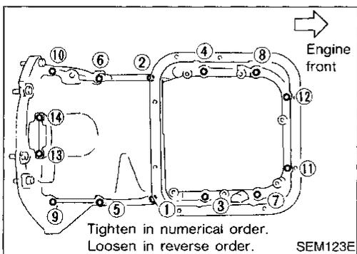
12. Remove aluminum oil pan nuts and bolts.
