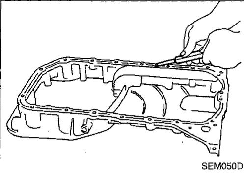
1. Use a scraper to remove old liquid gasket from mating surface of aluminum oil pan.
