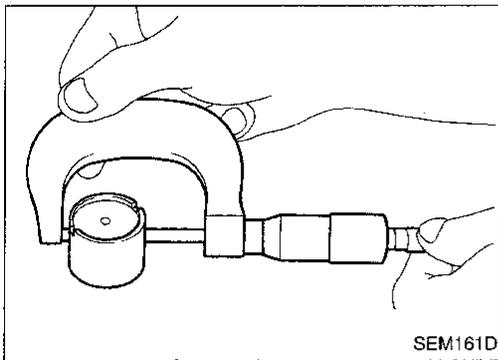
2. Check diameter of valve lifter and valve lifter guide bore.
