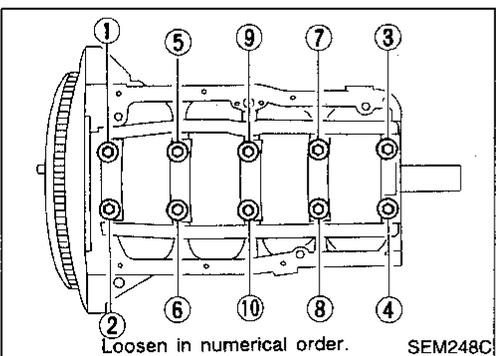
4. Remove main bearing cap and crankshaft.
