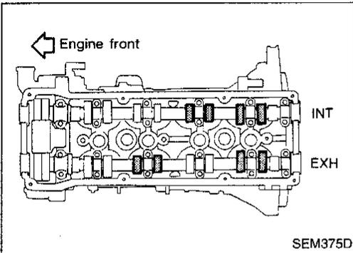
4. Turn crankshaft one revolution (360°) and align mark on crankshaft pulley with pointer.
