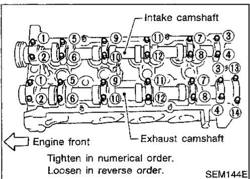
5. Install camshafts and camshaft brackets using the following procedure:
