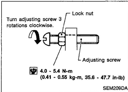
9. Turn adjusting screw 3 rotations clockwise.
