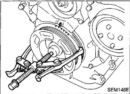
3. Remove crankshaft pulley.
