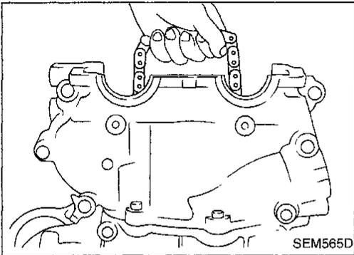
3. Install cam sprocket cover.
