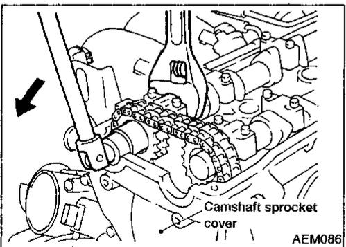
9. Remove cam sprocket.
