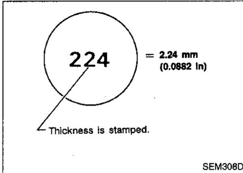
Shims are available in thicknesses from 1.96 mm (0.0772 in) to 2.68 mm (0.1055 in), in steps of 0.02 mm (0.0008 in).
