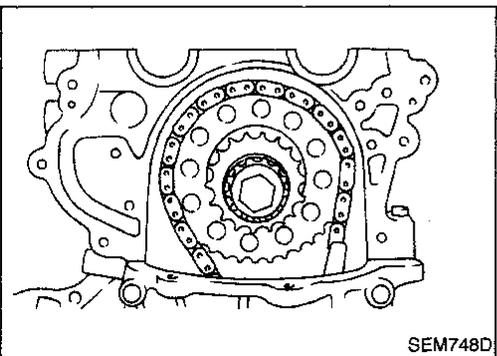
3. Install idler sprocket and lower timing chain.
