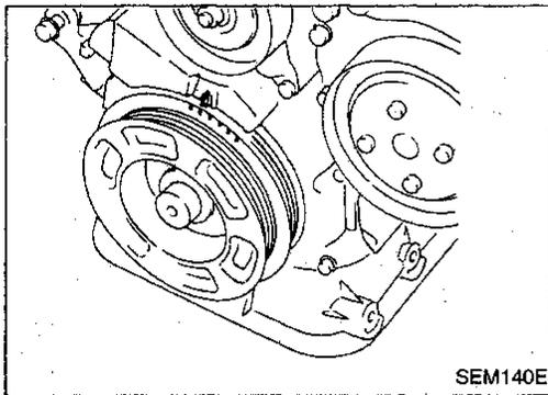
5. Set No. 1 piston at TDC on its compression stroke.
