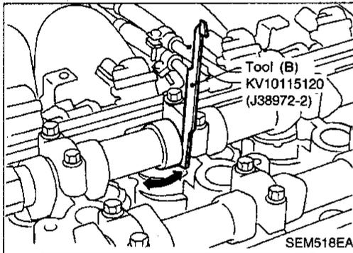
8. Install new shim using a suitable tool.
