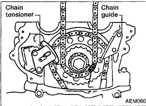
2. Install upper timing chain, chain tensioner and chain guide.
