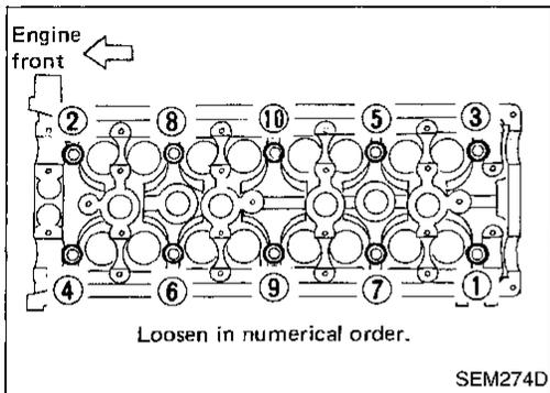
11. Loosen cylinder head bolts in numerical order.
