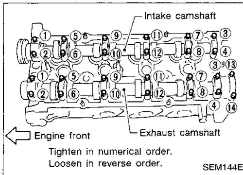
10. Remove camshaft brackets and camshafts.
