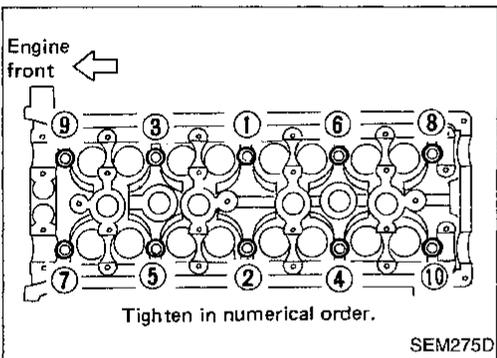
4. Tighten cylinder head bolts using the following procedure:
