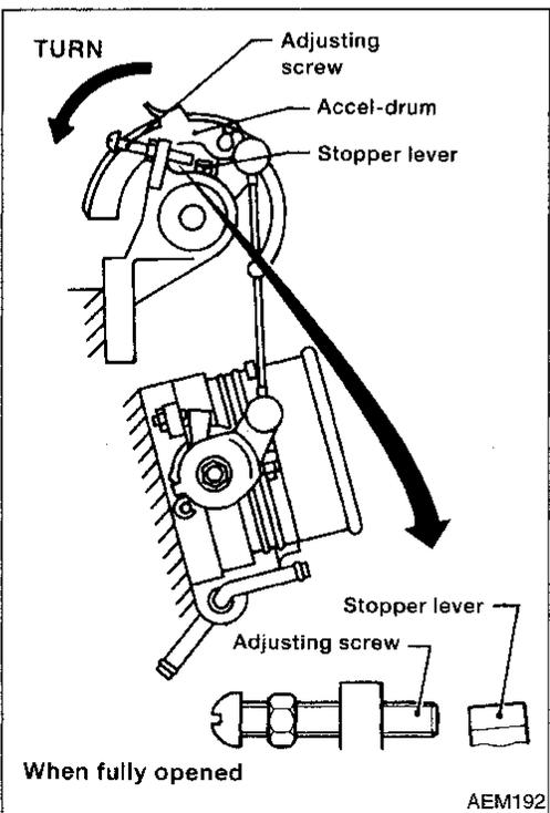
6. Manually turn accel-drum until throttle valve is fully open.
