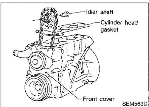
16. Remove cylinder head and cylinder head gasket.
