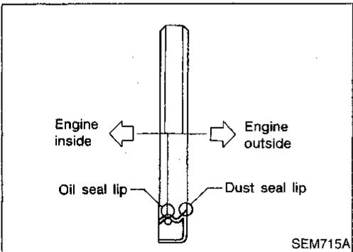
3. Install new oil seal in the direction shown.
