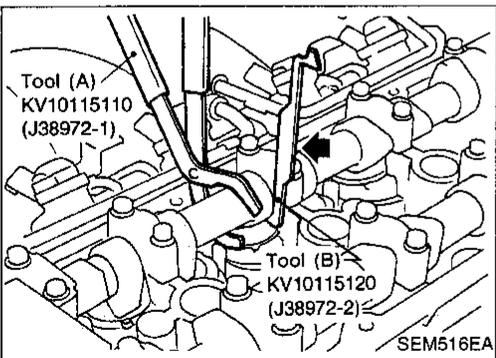
6. Remove adjusting shim using a small screwdriver and a magnetic finger.
