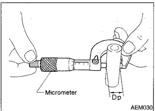
2. Measure outer diameter "Dp" of piston pin.
