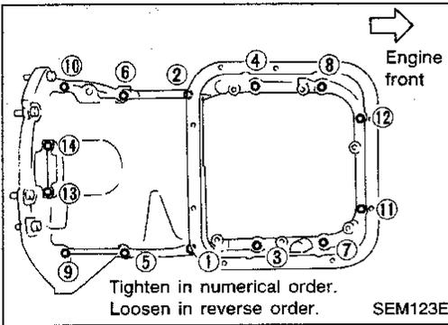
12. Remove aluminum oil pan nuts and bolts.
