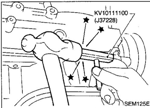
b. Slide Tool by tapping on the side of the Tool with a hammer.
