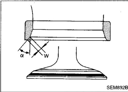
5. Cut or grind valve seat using suitable tool to the specified dimensions. Refer to SDS (EM-57).
