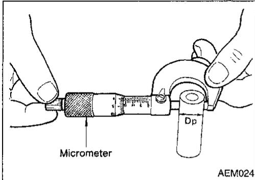
2. Measure outer diameter of piston pin "Dp".
