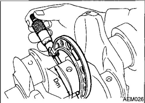
4. Measure outer diameter "Dm" of each crankshaft main journal.
