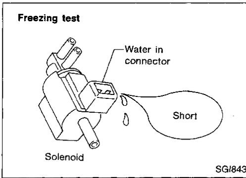
The customer may indicate the incident goes away after the car warms up (winter time). The cause could be related to water freezing somewhere in the wiring/electrical system.
