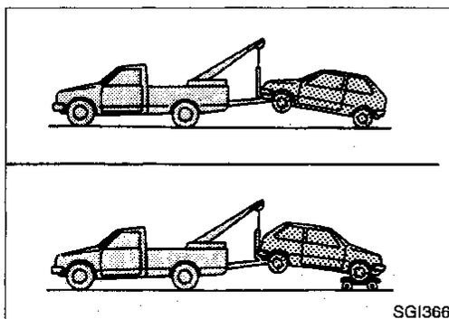
NISSAN recommends that vehicle be towed with the driving (front) wheels off the ground as illustrated.
