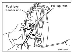
3. After fixing tabs are disengaged, slide fuel level sensor unit out in direction shown by the arrow.
