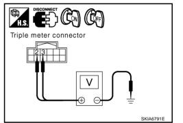
3. Check voltage between unified meter and A/C amp. harness connector terminals and ground.
