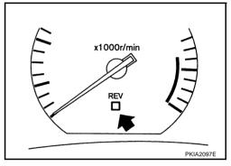
reaches the set figure. The figure of engine speed can changed between 2,000 and 8,000 rpm by pressing trip computer setting switch. Pressing the trip computer setting switch for less than approximately 1 second will add the figure by 100 rpm. If pressing for more than approximately 1 second, the figure will increase by 500 rpm.
