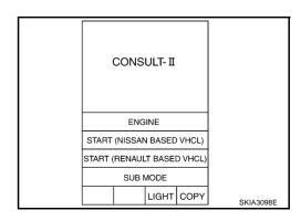
Touch "BCM" on "SELECT SYSTEM" screen. If "BCM" is not indicated, go to <u>GI-39</u>, "CONSULT-II Data Link Connector (DLC) Circuit".
