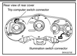
5. Remove screws (2) and remove rear cover.
