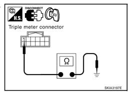
3. Check continuity between unified meter and A/C amp. harness connector M49 terminals 29 (B), 30 (B) and ground.
