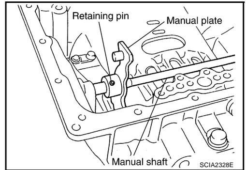
63. Remove manual shaft retaining pin with nippers.
