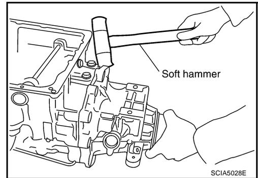
45. Remove rear extension assembly from transmission case. (With needle bearing)
