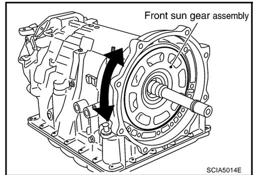
53. Install needle bearing to front sun gear.
