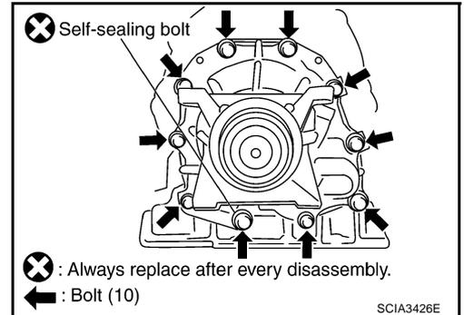
13. Install engine rear member. Refer to [AT-272, "Removal and Installation"](#) .
