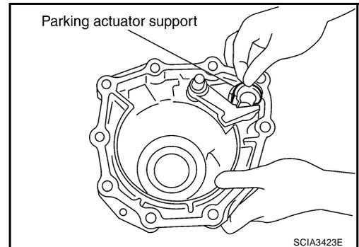
16. Remove parking pawl (with return spring) and pawl shaft from rear extension.
