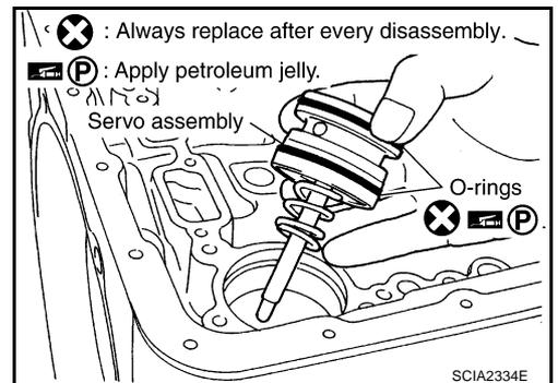
71. Remove return spring from servo assembly.
