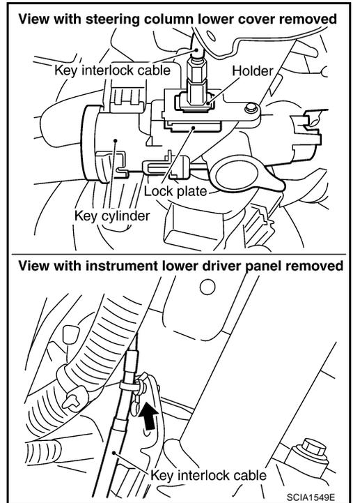
5. Insert interlock rod into adjuster holder.
