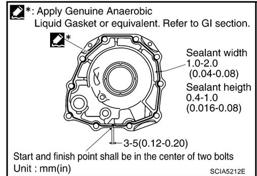
35. Install rear extension assembly to transmission case.
