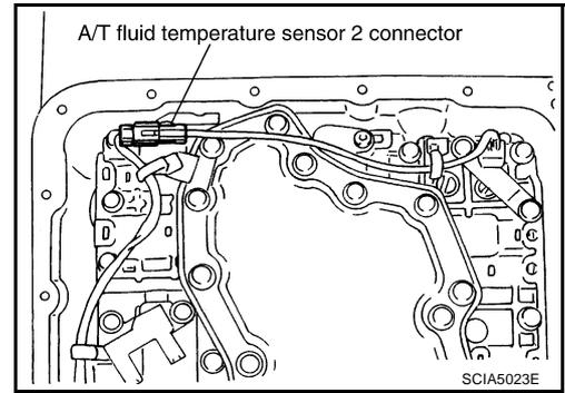
11. Straighten terminal clips to free terminal cord assembly and A/T fluid temperature sensor 2 harness.
