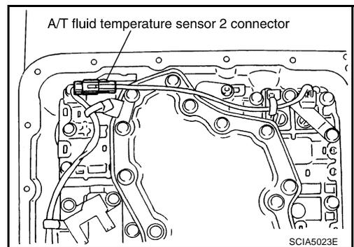
11. Securely fasten terminal cord assembly and A/T fluid temperature sensor 2 harness with terminal clips.
