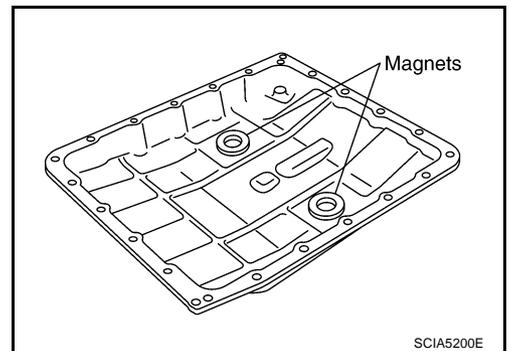
15. Install oil pan to transmission case.
