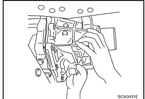
6. Tighten rear extension assembly mounting bolts to specified torque.
