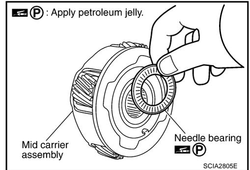
47. Install mid carrier assembly in rear carrier assembly.
