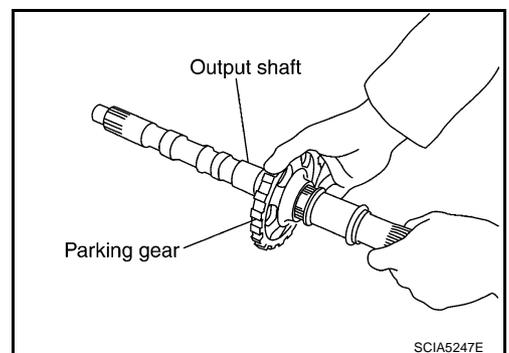
32. Install output shaft in transmission case.
