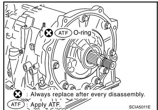
7. Install converter housing to transmission case.
