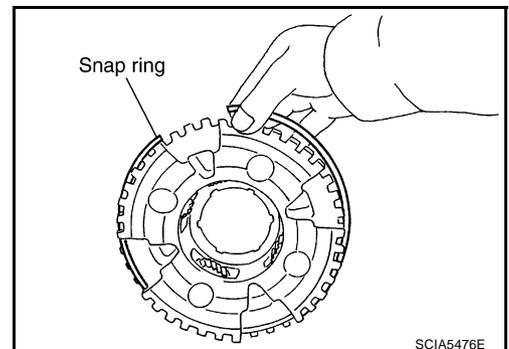
4. Disassemble input clutch assembly.
