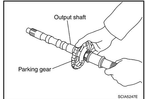
8. Install output shaft to transmission case.
