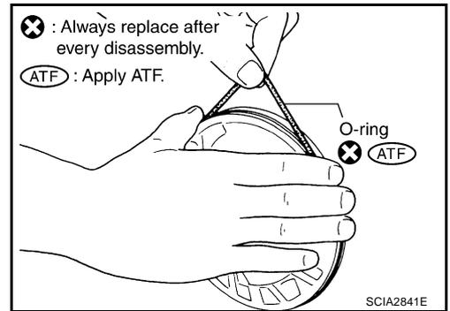
4. Remove O-ring from oil pump cover.
