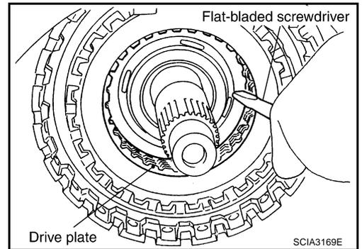
41. Install high and low reverse clutch hub, mid sun gear assembly and rear sun gear assembly as a unit.
