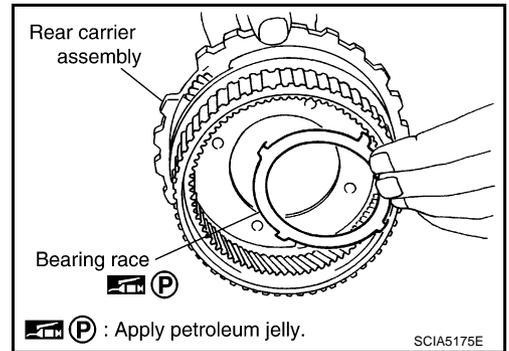
21. Remove needle bearing from rear carrier assembly.
