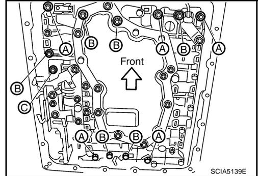
9. Tighten bolt 1, 2 and 3 temporarily to prevent dislocation. After that tighten them in order (1 → 2 → 3), and then tighten other bolts.
