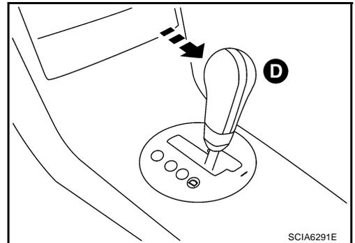
5. Depress brake pedal. (Stop lamp switch signal "ON".)
