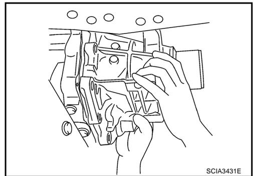
10. Remove bearing race from output shaft.
