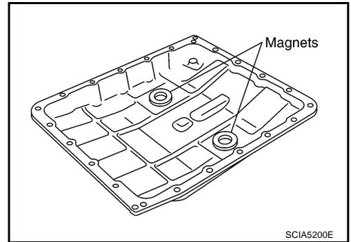
17. Install oil pan to transmission case.
