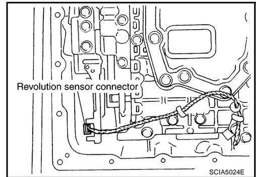
13. Straighten terminal clips to free revolution sensor harness.
