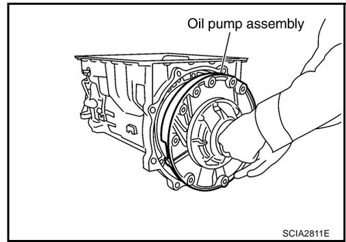
4. Apply recommended sealant (Genuine RTV Silicone Sealant or equivalent. Refer to [GI-47, "Recommended Chemical Products and Sealants"](#) .) to oil pump assembly as shown in the figure.
