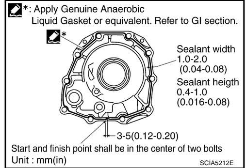
5. Install rear extension assembly to transmission case. (With needle bearing.)
