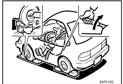
4. Engine start, apply foot brake, and place selector lever in "D" position.
