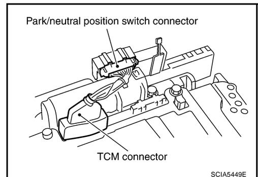
2. Install A/T assembly harness connector from control valve with TCM.
