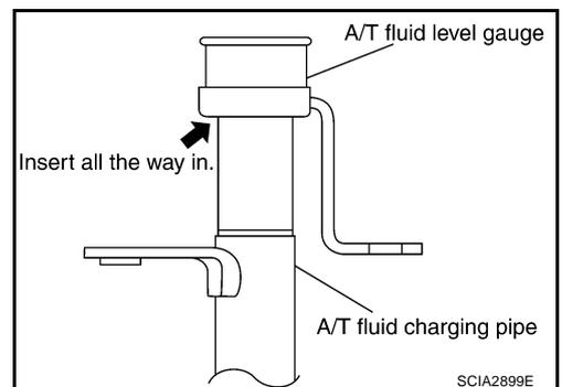
9. Install the removed A/T fluid level gauge in the A/T fluid charging pipe.
