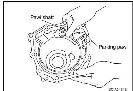
4. Install parking actuator support to rear extension.
