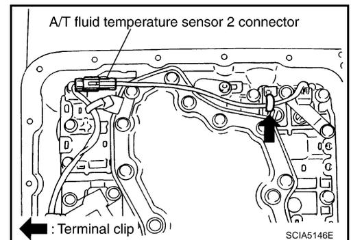
8. Remove A/T fluid temperature sensor 2 with bracket from control valve with TCM.
