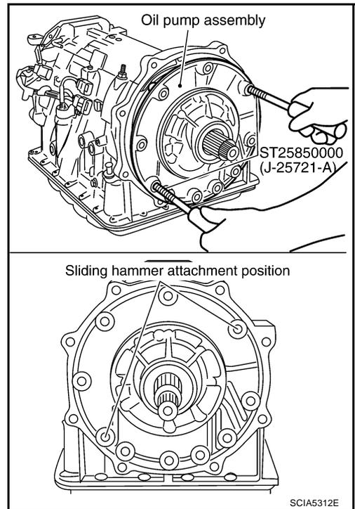
8. Remove O-ring from oil pump assembly.
