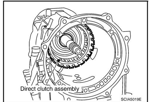
25. Remove needle bearing from drum support.
