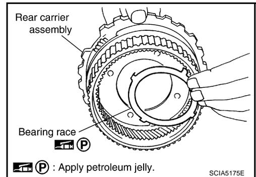
44. Install rear carrier assembly in direct clutch drum.
