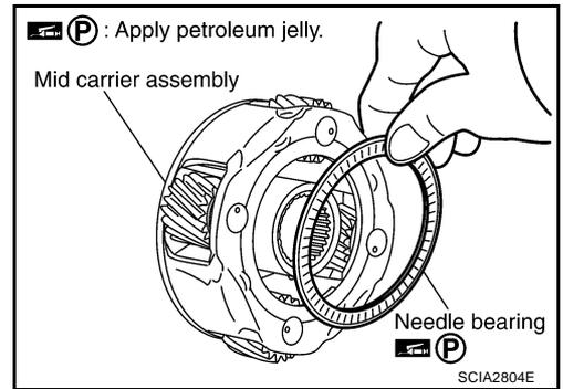
46. Install needle bearing (front side) to mid carrier assembly.
