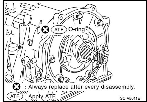
6. Remove tightening bolts for oil pump assembly and transmission case.
