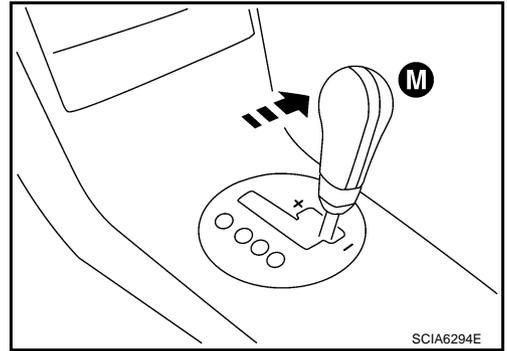
2. Release brake pedal. (Stop lamp switch signal "OFF".)
