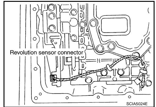
13. Securely fasten revolution sensor harness with terminal clips.
