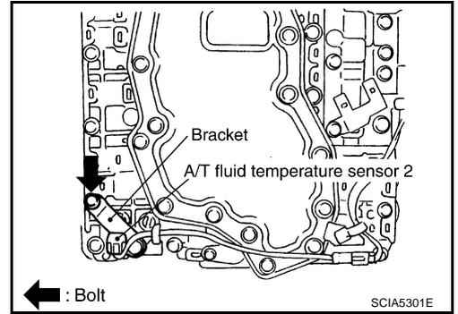
38. Remove bracket from A/T fluid temperature sensor 2.
