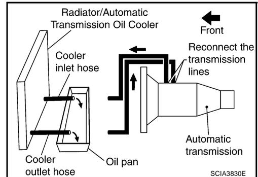
5. Insert the extension adapter hose of a can of Transmission Cooler Cleaner (Nissan P/N 999MP-AM006) into the cooler outlet hose.
