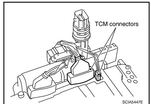
41. Remove A/T assembly harness connector from control valve with TCM using a flat-bladed screwdriver.
