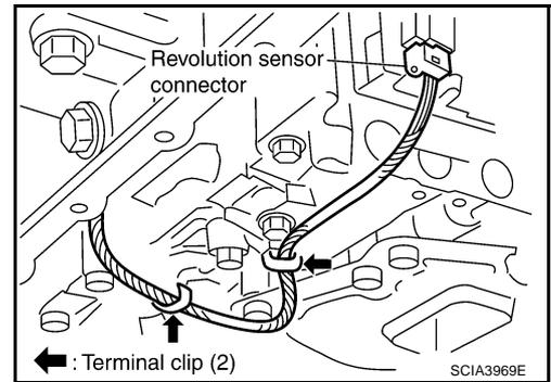
15. Remove revolution sensor from transmission case.
