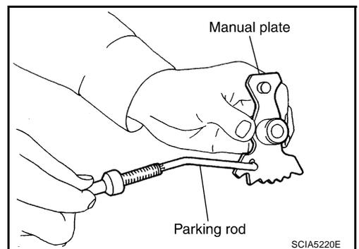
66. Remove manual shaft from transmission case.
