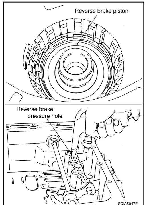
61. Remove D-rings from reverse brake piston.
