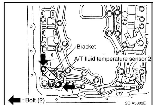
3. Connect A/T fluid temperature sensor 2 connector.
