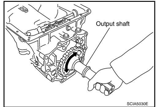
48. Remove parking gear from output shaft.
