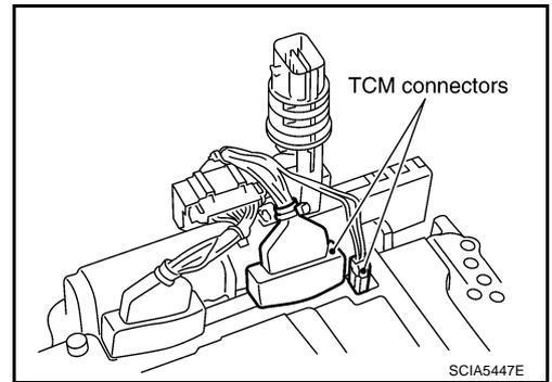
4. Install O-ring in A/T assembly harness connector.
