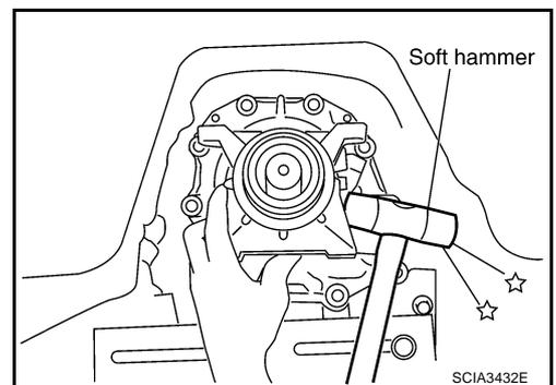
12. Remove rear extension assembly from transmission case. (With needle bearing.)
