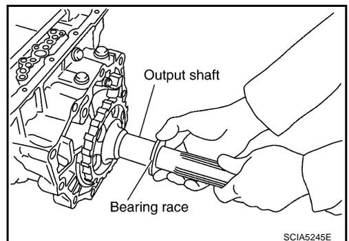
11. Remove output shaft from transmission case by rotating left/right.
