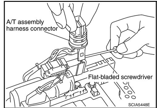
21. Disconnect TCM connector and park/neutral position switch connector.
