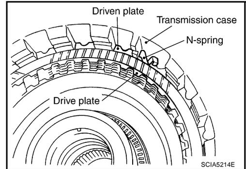
55. Remove reverse brake drive plates, driven plates and dish plate from transmission case.
