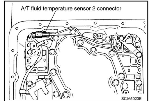
7. Straighten terminal clip to free A/T fluid temperature sensor 2 harness.
