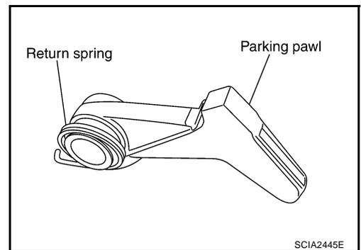
3. Install parking pawl (with return spring) and pawl shaft to rear extension.
