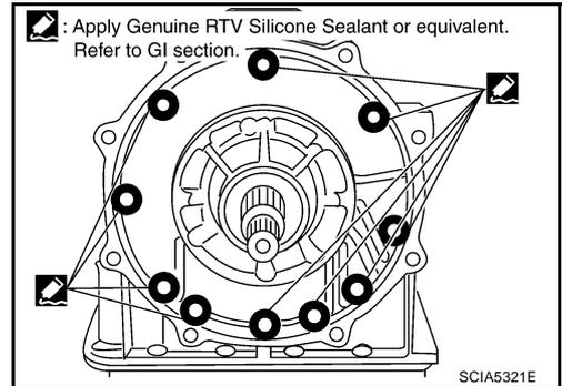
5. Tighten oil pump mounting bolts to specified torque.
