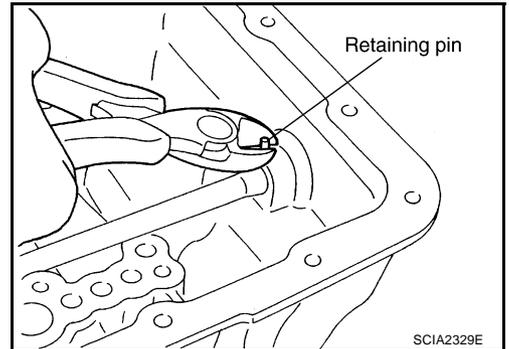
64. Remove manual plate (with parking rod) from manual shaft.
