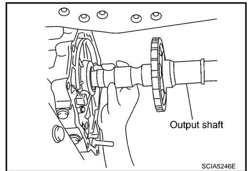
9. Install bearing race to output shaft.
