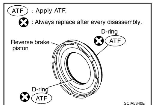
13. Install reverse brake piston in transmission case.
