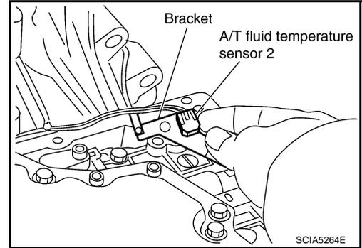
f. Install A/T fluid temperature sensor 2 (with bracket) in control valve with TCM.
