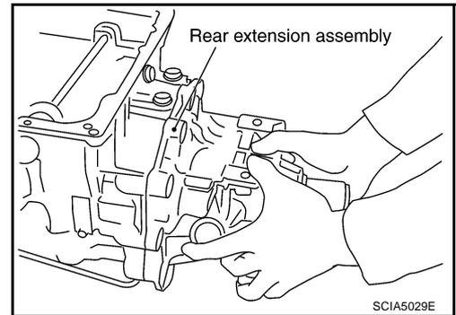
36. Tighten rear extension assembly mounting bolts to specified torque.
