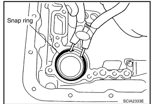
70. Remove servo assembly (with return spring) from transmission case.
