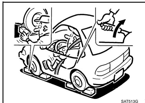
5. Start the engine, then measure the line pressure at both idle and the stall speed.
