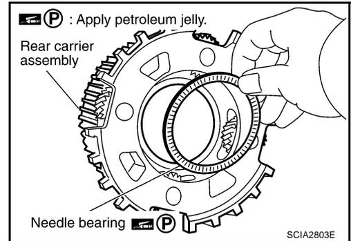
43. Install bearing race in rear carrier assembly.
