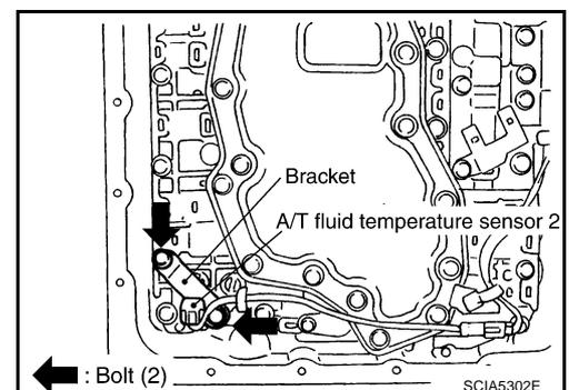
9. Remove bracket from A/T fluid temperature sensor 2.
