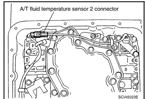
4. Securely fasten A/T fluid temperature sensor 2 harness with terminal clip.
