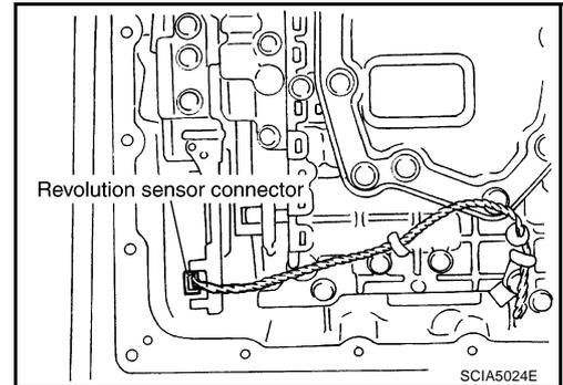
34. Straighten terminal clips to free revolution sensor harness.
