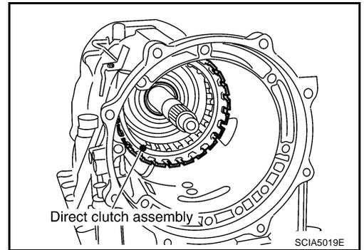
39. Install high and low reverse clutch assembly in direct clutch.
