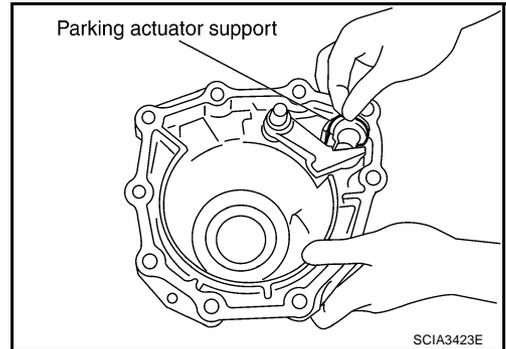
74. Remove parking pawl (with return spring) and pawl shaft from rear extension.
