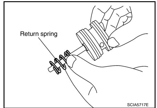
10. Install servo assembly in transmission case.
