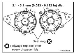
Install new collared O-rings in front timing chain case oil hole (left and right sides).
