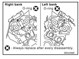
32. Remove O-rings from cylinder block.
