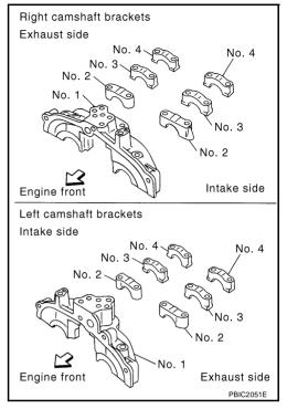
• Install camshaft brackets (No. 2 to 4) aligning the stamp marks as shown in the figure.
