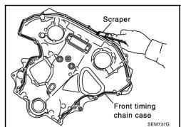
• Remove old liquid gasket from bolt hole and thread.
