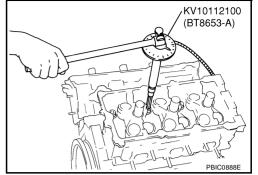
4. After installing cylinder head, measure distance between front end faces of cylinder block and cylinder head (left and right banks).
