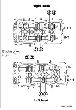
d. Rotate crankshaft by 240 degrees clockwise (when viewed from engine front) to align No. 5 cylinder at TDC of compression stroke.
