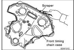
• Remove old liquid gasket from bolt hole and thread.
