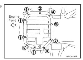
b. Insert seal cutter [SST] between oil pan (upper) and oil pan (lower).
