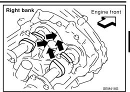
Use feeler gauge, measure the clearance between valve lifter and camshaft.
