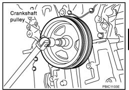
Place suitable puller tab on holes of crankshaft pulley, and pull crankshaft pulley through.
