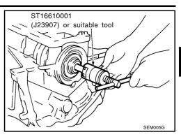
13. Remove rear oil seal retainer.
