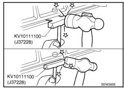
c. Slide seal cutter by tapping on the side of the tool with hammer. Remove oil pan (lower).
