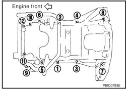
24. Remove O-rings from bottom of cylinder block and oil pump.
