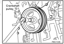
c. Place suitable puller tab on holes of crankshaft pulley, and pull crankshaft pulley through.
