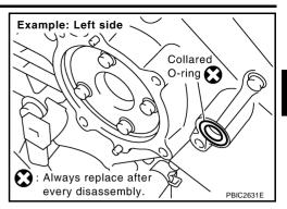
d. Being careful not to move seal ring from the installation groove, align dowel pins on front timing chain case with the holes to install intake valve timing control covers.
