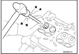
3. Using valve guide reamer (commercial service tool), ream cylinder head valve guide hole.
