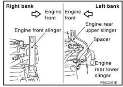
To protect rocker cover against damage caused by tilting of engine slinger, insert spacer between cylinder head and engine rear lower slinger, in direction shown in the figure.
