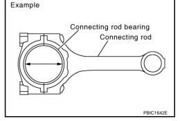
If the calculated value exceeds the limit, select proper connecting rod bearing according to connecting rod big end diameter and crankshaft pin journal diameter to obtain the specified bearing oil clearance. Refer to <u>EM-125</u>, "HOW TO SELECT CONNECTING ROD BEARING".
