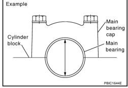
If the clearance exceeds the limit, select proper main bearing according to main bearing inner diameter and crankshaft main journal diameter to obtain the specified bearing oil clearance. Refer to <u>EM-126</u>, "HOW TO SELECT MAIN BEARING".
