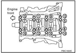
Turn all bolts another 90 to 95 degrees clockwise [Target: 90 degrees (Angle tightening)].
