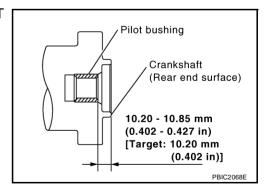
Press-fit pilot converter with its chamfer facing crankshaft as shown in the figure. (A/T models)
