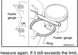
Piston Press-fit Feeler gauge Piston ring 0 Piston ring Measuring point PBIC0118F
