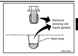
35. Use scraper to remove all traces of liquid gasket from water pump cover, chain tensioner cover and intake valve timing control covers.
