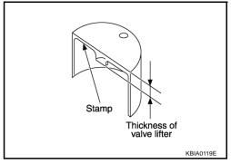
Available thickness of valve lifter: 27 sizes with range 7.88 to 8.40 mm (0.3102 to 0.3307 in) in steps of 0.02 mm (0.0008 in) (when manufactured at factory). Refer to EM-144, "Available Valve Lifter".
