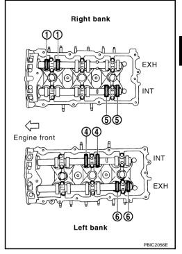
3. For measured value are out of the standard, perform adjustment. Refer to EM-87, "ADJUSTMENT".
