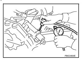
Use compression gauge whose picking up end inserted to spark plug hole is smaller than 20 mm (0.79 in) in diameter.
