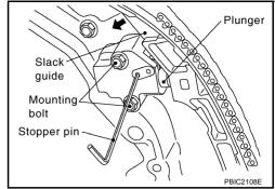
26. Remove internal chain guide, tension guide and slack guide.
