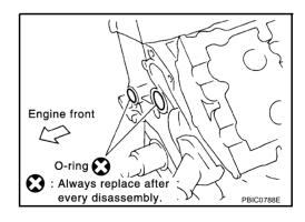
b. Install new O-rings to cylinder head.
