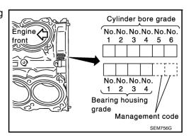
"Main Bearing Selection Table" columns correspond to journal diameter grade on front side of crankshaft.
