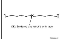
• Do not make a bypass connection to repaired area. (If it is done, branch part will be removed and characteristics of twisted wire will be lost.)
