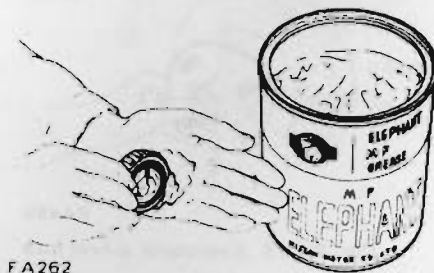
Fig. FA-18 Filling bearing cone with grease
