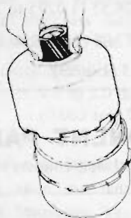
Fig. AT-73 Installing connecting shell
