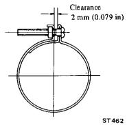
Fig. ST-44 Tightening boot clamp
