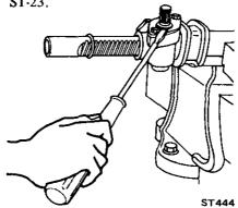
Fig. ST-23 Removing oil seal
