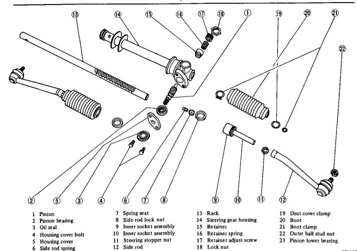
Fig. ST-26 Rack-and-pinion and side rod components
