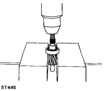
Fig. ST-25 Pressing pinion bearing out of pinion shaft
