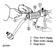
Fig. ST-20 Removing clamps
