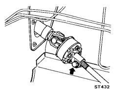
Fig. ST-4 Removing rubber coupling
