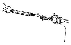
Fig. ST-38 Measuring rack force to pull
