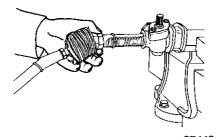
Fig. ST-21 Disconnecting side rod assembly
