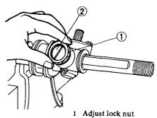
2 Retainer adjust screw Fig. ST-22 Removing adjust lock nut
