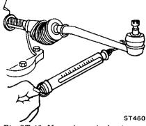
Fig. ST-42 Measuring swinging torque
