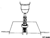
Fig. ST-29 Pressing bearing onto pinion gear
