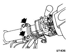
Fig. ST-14 Removing steering lock securing screws
