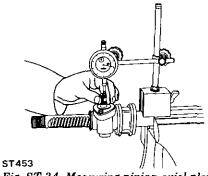
Fig. ST-34 Measuring pinion axial play
