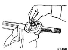
Fig. ST-31 Inserting pinion assembly
