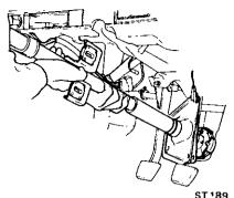
Fig. ST-7 Drawing out steering column assembly
