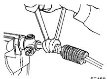
Fig. ST-41 Tightening lock nut
