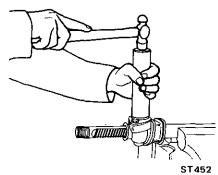
Fig. ST-33 Fitting oil seal
