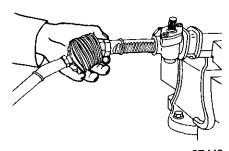
Fig. ST-39 Fitting side rod assembly to rack
