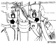
Fig. ST-6 Removing column clamp securing bolts
