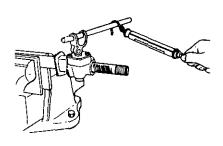
ST456 Fig. ST-37 Measuring pinion rotary torque
