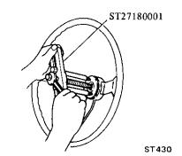
Fig. ST-2 Removing steering wheel
