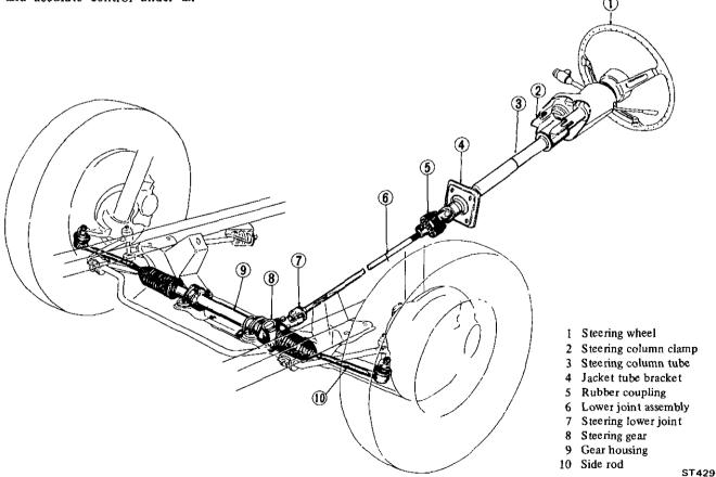
Fig.ST-1 Structural view of steering system
