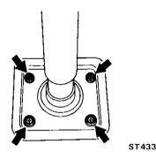
Fig. ST-5 Removing jacket tube bracket securing bolts
