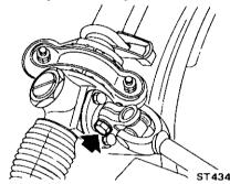
Fig. ST-8 Loosening nut securing lower joint to pinion
