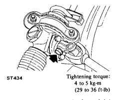
Fig. ST-17 Disconnecting lower joint from pinion
