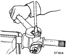
Fig. ST-35 Locking retainer lock nut
