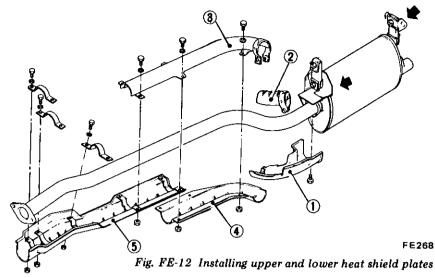
3. Upper and lower catalytic converter heat shield plates.
