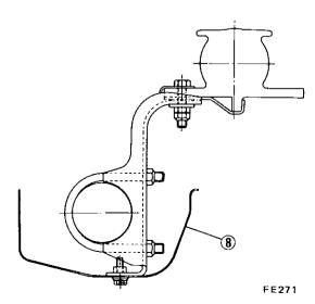
Fig. FE-15 Exhaust front tube mounting bracket
