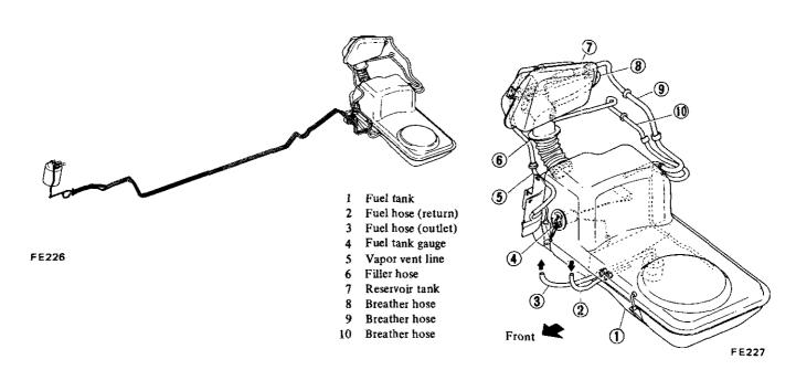
Fig. FE-5 Fuel tank and fuel line
