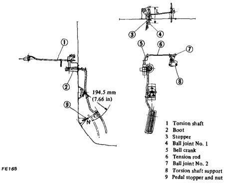
Fig. FE-4 Accelerator linkage setting
