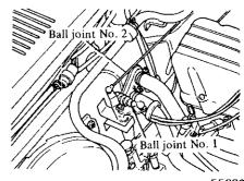
Fig. FE-3 Disconnecting ball joint rods
