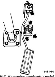
Fig. FE-2 Removing accelerator pedal
