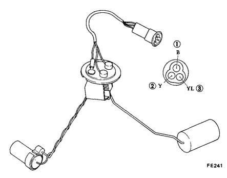
Fig. FE-7 Fuel tank gauge
