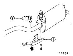
Fig. FE-11 Installing upper heat shield plate
