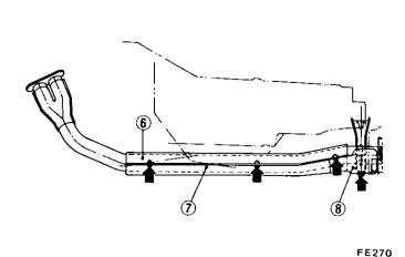
Fig. FE-14 Exhaust front tube heat shield plate
