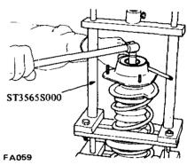
Fig. FA-27 Removing self-locking nut
