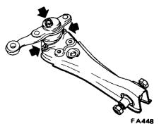
Fig. FA-41 Removing knuckle arm
