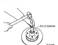
Fig. FA-18 Installing wheel bearing outer race
