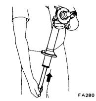
Fig. FA-36 Bleeding air from strut
