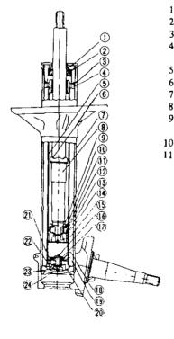
1 Gland packing assembly 12 Piston ring 2 Oil seal Valve plate 3 O-ring Piston body Piston rod guide 15 Nut assembly 16 Rolt Cylinder 17 Distance collar Rebound stopper Spring retainer 7 Strut-outer casing 19 Check valve spring Piston rod 20 Bottom valve body Check valve spring 21 Check valve plate retainer 22 Valve plate 10 Check valve spring 23 Nut 11 Check valve plate
