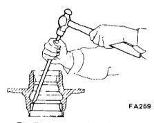
Fig. FA-13 Removing wheel bearing outer race
