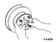
Fig. FA-12 Removing wheel hub
