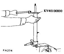
Fig. FA-34 Tightening gland packing
