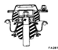
Fig. FA-37 Strut mounting bearing greasing point
