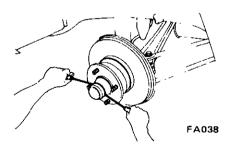
Fig. FA-11 Removing hub cap
