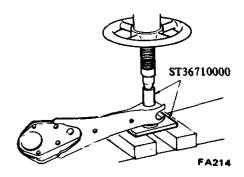
Fig. FA-42 Removing transverse link bushing
