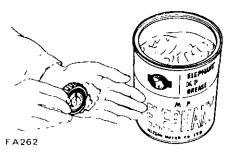
Fig. FA-20 Filling bearing cone with
