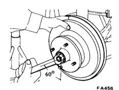
Fig. FA-3 Loosen wheel bearing lock nut 60°
