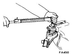
Fig. FA-45 Tightening knuckle arm castle nut
