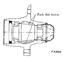
Fig. FA-19 Lubricating points of wheel hub
