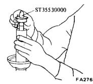
Fig. FA-32 Installing gland packing
