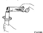
Fig. FA-31 Filling outer casing with fluid
