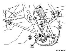
Fig. FA-39 Removing stabilizer and compression rod
