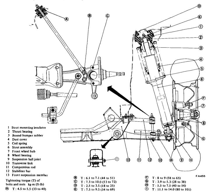
Fig. FA-1 Front axle and suspension assembly
