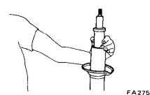
Fig. FA-29 Removing piston rod and cylinder
