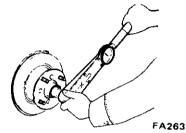
Fig. FA-2 Tightening wheel bearing lock nut
