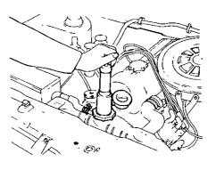
Fig. CO-11 Testing radiator pressure
