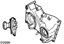
Fig. CO-2 Water pump and front
