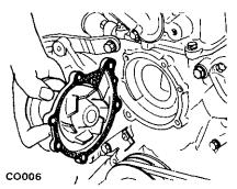
Fig. CO-3 Removing water pump
