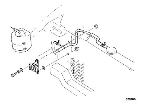
Fig. CO-14 Installing reservoir tank
