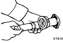
Fig. CO-10 Testing radiator cap
