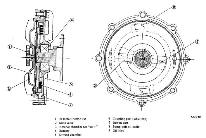
Fig. CO-4 Cross-sectional view of Tem-coupling
