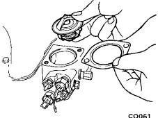
Fig. CO-6 Removing thermostat
