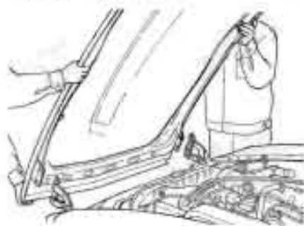
Fig. ER-1 Removing hood
