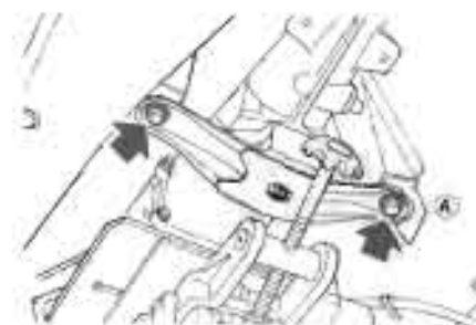
Fig. ER-8 Removing propeller shaft
