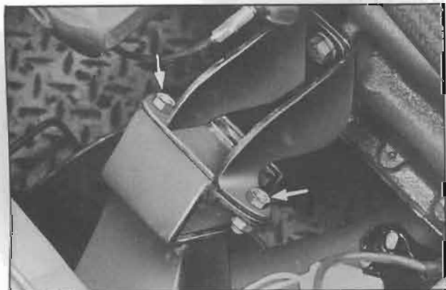
Fig. FA-7 Removing engine mounting bolts
