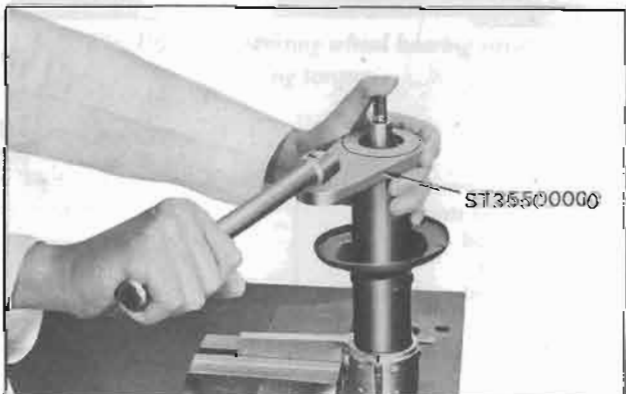
Fig. FA-31 Removing gland packing
