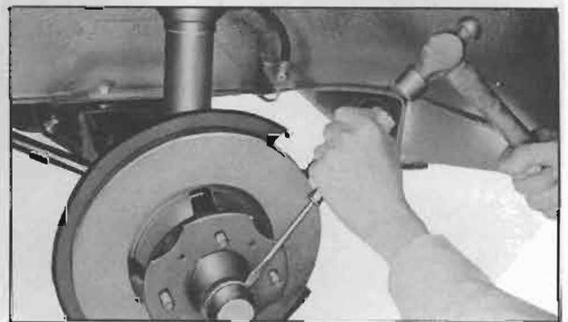
Fig. FA-14 Removing hub cap
