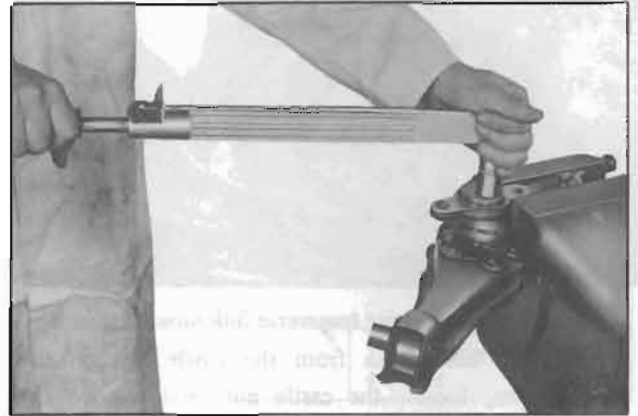
Fig. FA-48 Tightening knuckle arm castle nut
