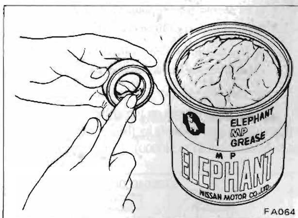
Fig. FA-33 Greasing strut mounting bearing
