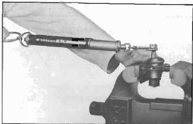
Fig. FA-47 Measuring ball joint shaking torque
