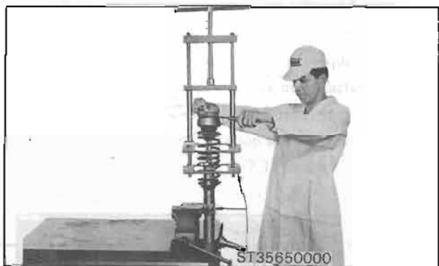
Fig. FA-30 Removing self-locking nut
