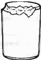
d) Cracked roller
