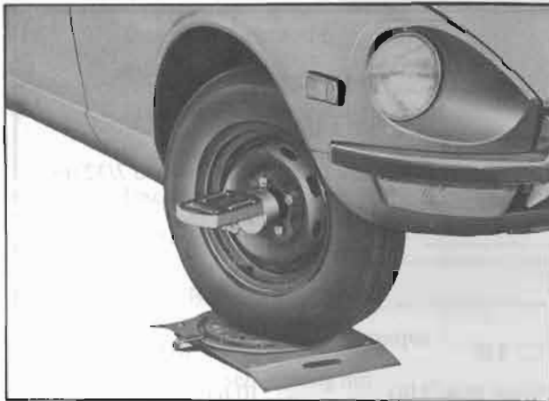
Fig. FA-49 Measuring steering angle, camber and caster
