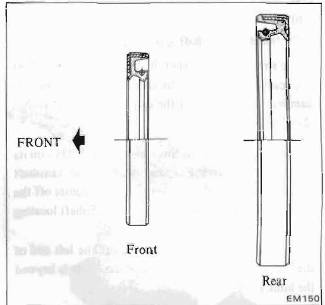
Fig. EM-67 Oil seal of crankshaft
