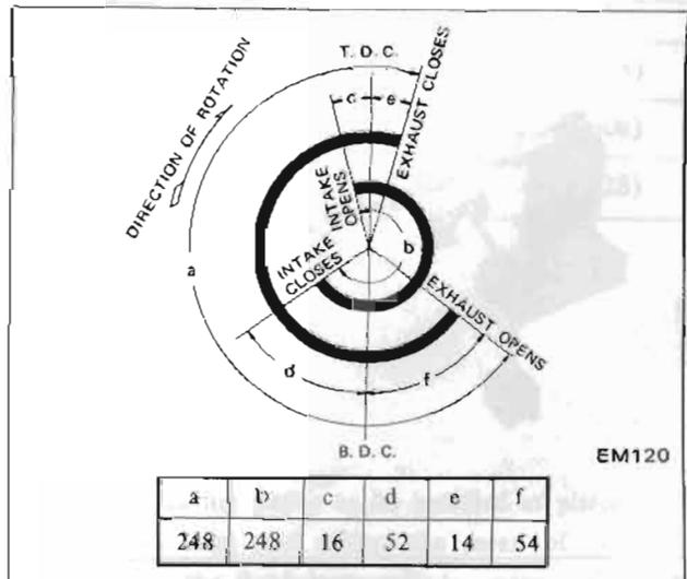
Fig. EM-38 Valve timing diagram
