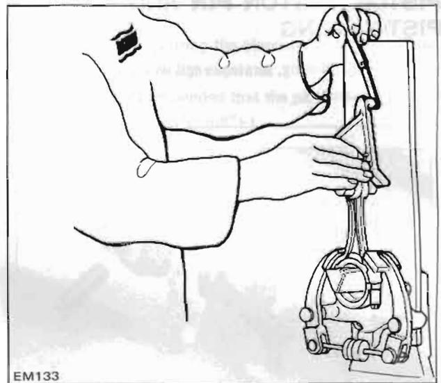
Fig. EM-51 Connecting rod alignment
