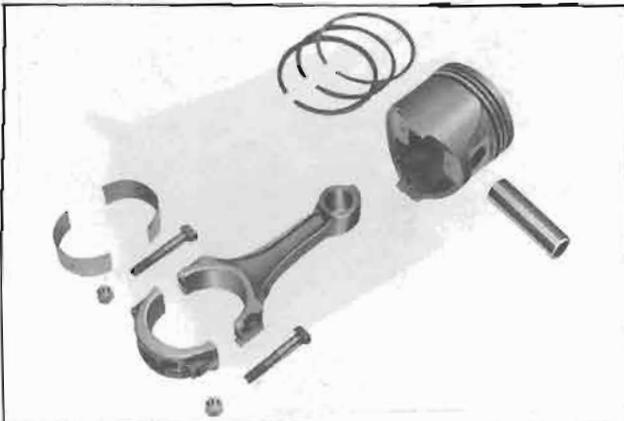
*Fig. EM-4 Piston and connecting rod*
