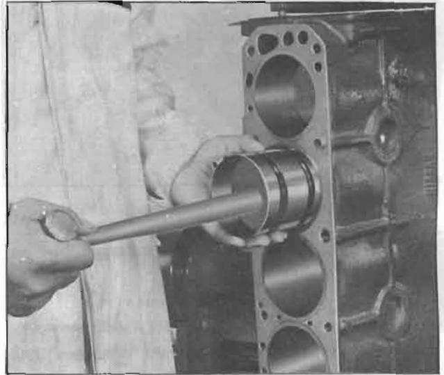
Fig. EM-81 Piston-rod assembly installation
