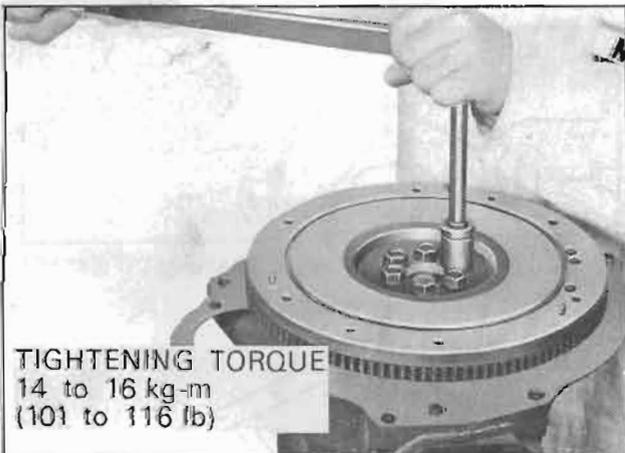
Fig. EM-80 Flywheel installation
