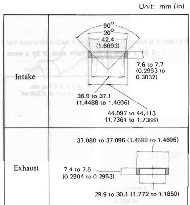
Fig. EM-36 Standard valve seat insert
