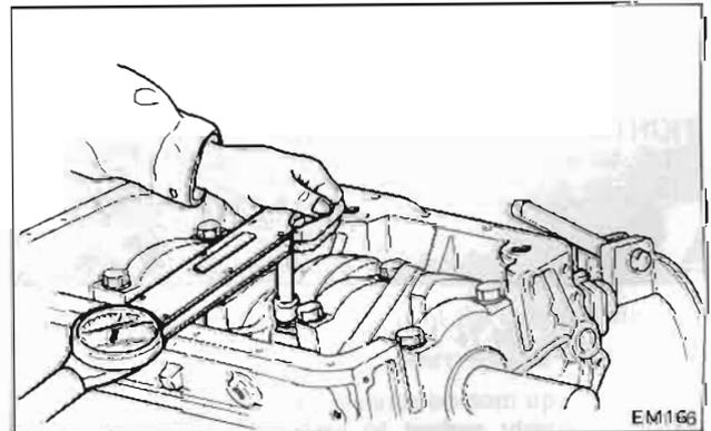
Fig. EM-82 connecting rod cap installation
