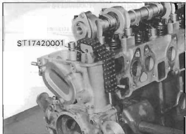
*Fig. EM-12 Camshaft drive sprocket removal*
