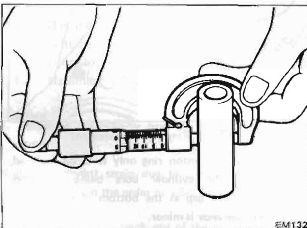
Fig. EM-50 Measuring piston pin diameter
