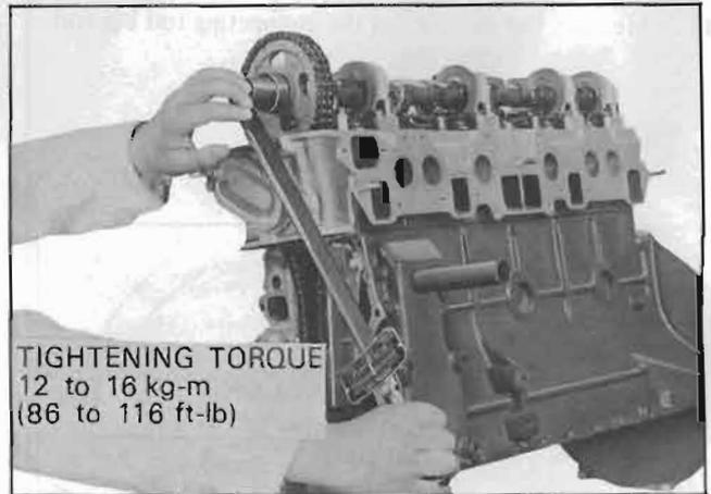
Fig. EM-89 Fuel pump cam installation
