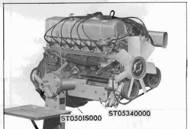
Fig. EM-10 The engine on the engine stand
