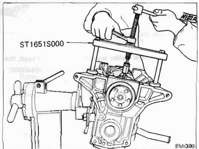
Fig. EM-17 Rear main bearing cap removal
