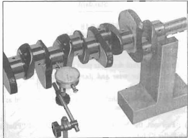
Fig. EM-54 Crankshaft bend check
