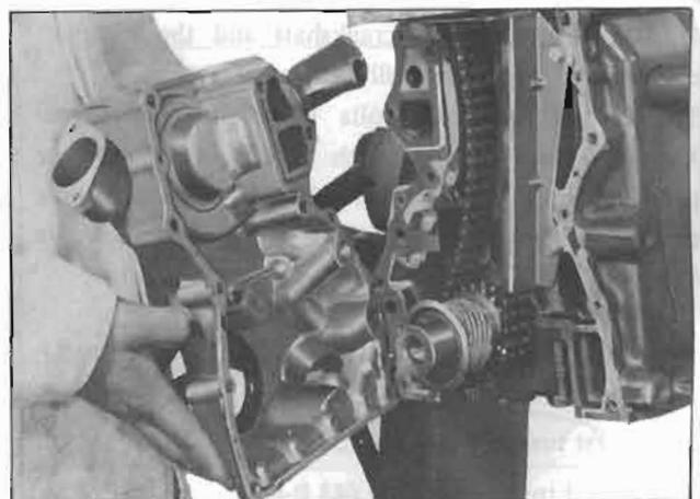
Fig. EM-90 Front cover installation
