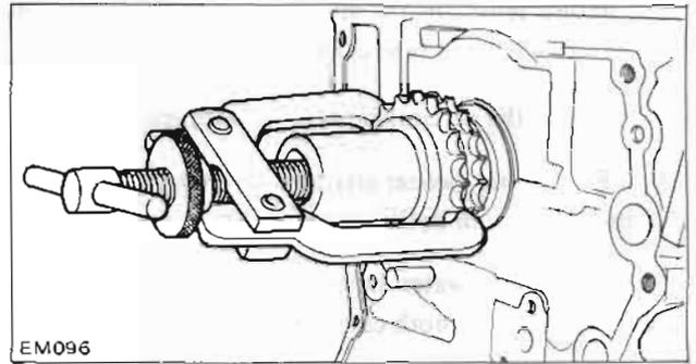
Fig. EM-15 Chain drive sprocket removal
