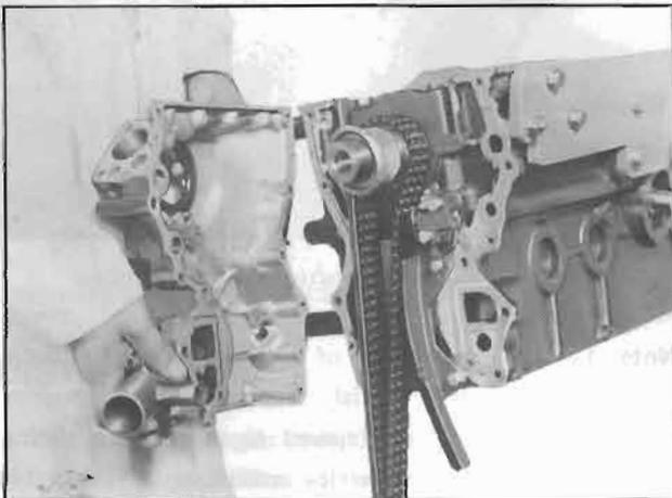
Fig. EM-14 Engine front cover removal
