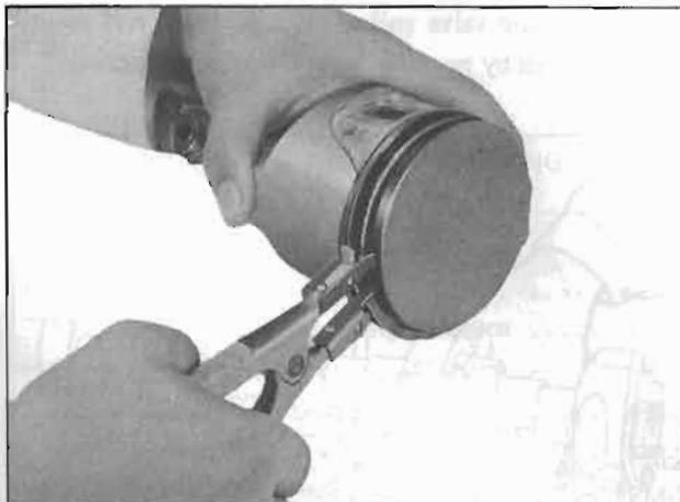
*Fig. EM-20 Piston ring removal*
