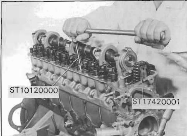
Fig. EM-13 Cylinder head removal
