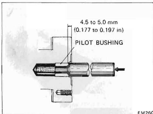
Fig. EM-57 Press-fitting new pilot bushing
