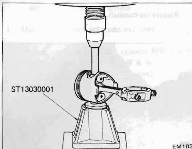
*Fig. EM-21 Piston pin removal*
