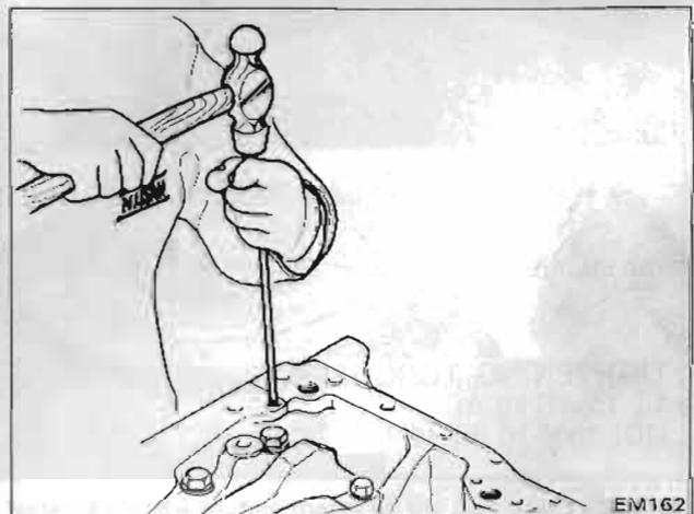
Fig. EM-78 Side oil seal installation
