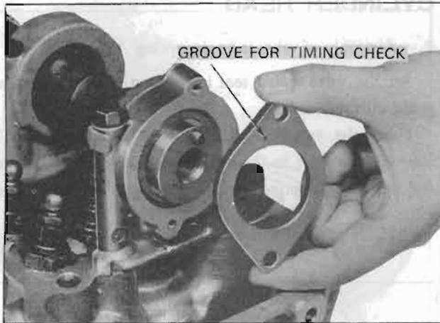
Fig. EM-72 Camshaft locating plate installation
