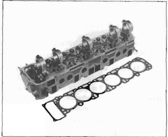
*Fig. EM-5 Cylinder head*
