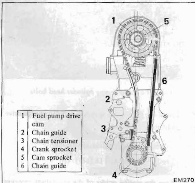
Fig. EM-88 Timing chain installation
