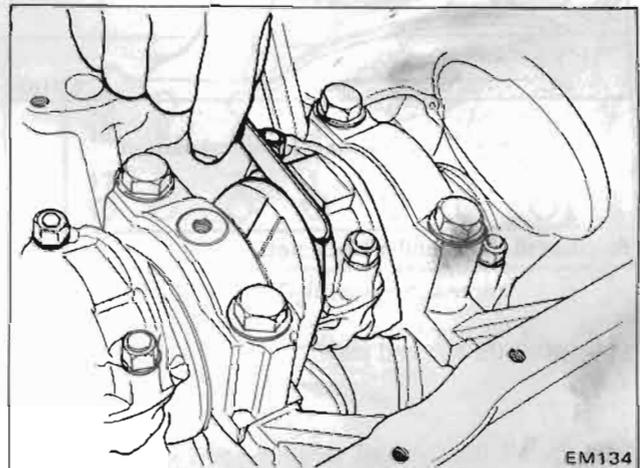
Fig. EM-77 Camshaft end play check
