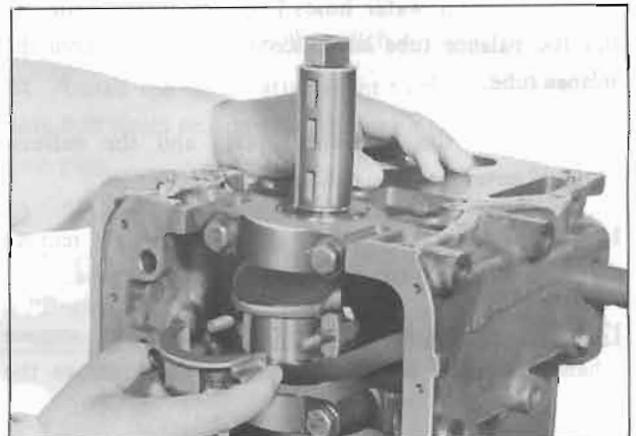
Fig. EM-16 Piston and connecting rod assembly removal
