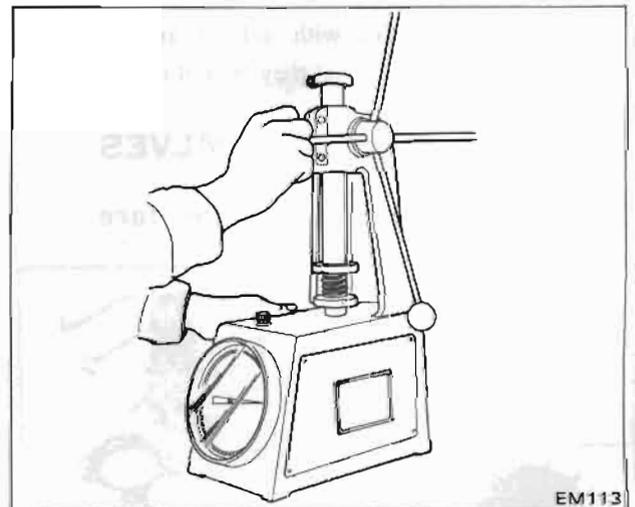
Fig. EM-31 Valve spring test
