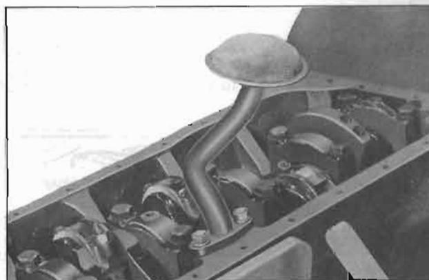
Fig. EM-93 Oil strainer installation
