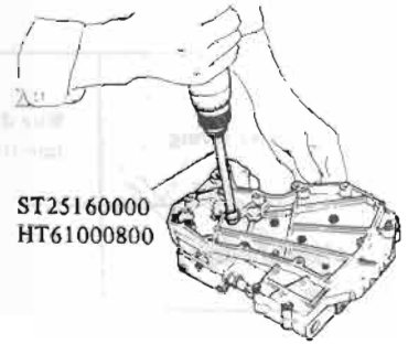
Fig. AT-108 Installing valve body
