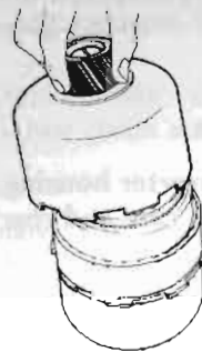
Fig. AT-73 Installing connecting shell
