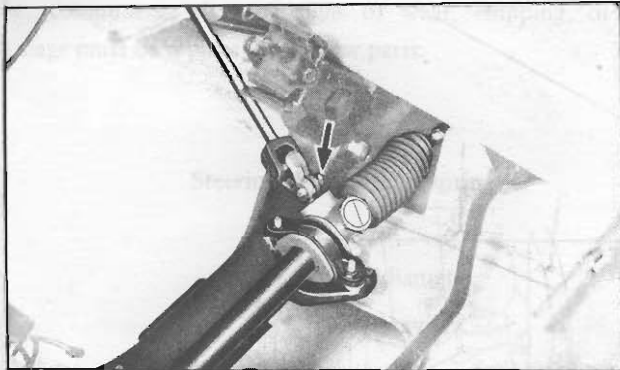
Fig. ST-13 Disconnecting lower joint from pinion
