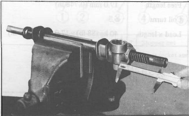
Fig. ST-26 Measuring protruding portion of rack
