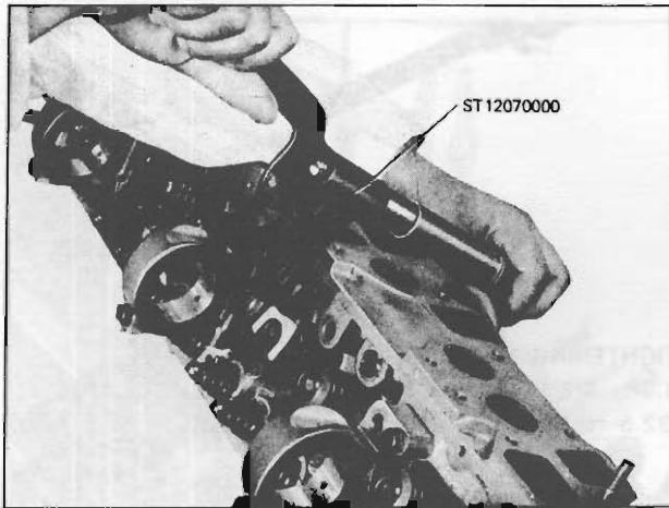
Fig. EM-69 Valve installation
