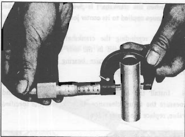
Fig. EM-56 Measuring piston pin diameter
