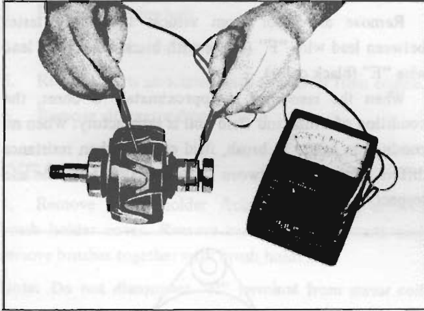
Fig. EE-41 Testing rotor coil for grounding
