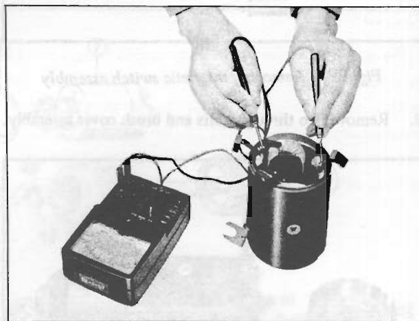
Fig. EE-12 Field coil test for continuity
