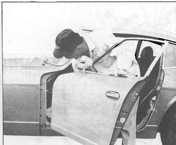
Fig. BF-19 Removing the door
