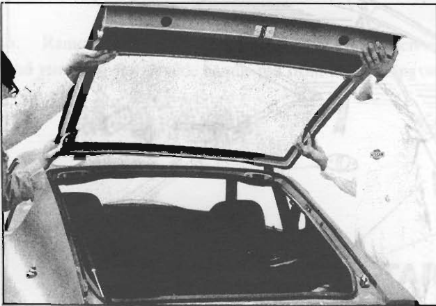
Fig. BF-38 Removing tail gate
