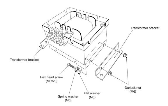
7. Refit the new Transformer using 2off hex head screws (M6x20), with flat and spring washers, and 2off wood screws (No10x¾).
