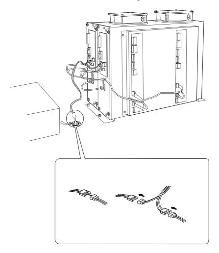
10. Refit the existing connectors to the I/O Boards and Front Cover Boards.
