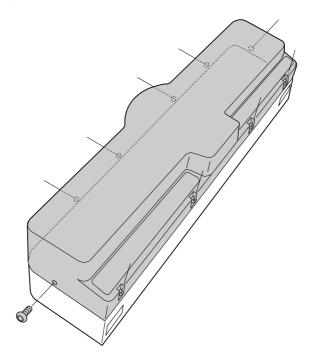
2. Remove 2off pozi head screw (M4x12) and remove the Top Bracket. (This part is no longer required).
