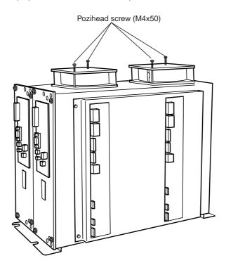
THESE FANS <u>MUST</u> BE FITTED TO THE NEW GAME PCB OR IRREPERABLE DAMAGE WILL BE CAUSED TO THE NEW GAME PCB.
