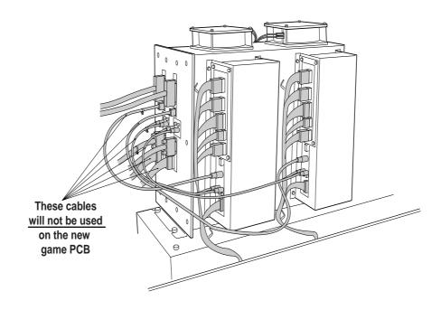
2. Remove the 2off pozi head screws (M6x25) from the right hand end of the Game PCB. slacken the 2off pozi head screws (M6x25) on the left hand end and remove the Game PCB.
