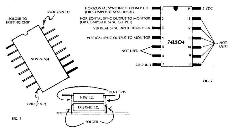
CURE 2: Used for Wells-Gardner Video-Sync boards with positive sync connections only. (Vertical mount board 85x14 OB.
