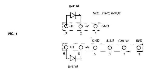
CURE 3: Join negative sync inputs J2 and J3 together with a jumper. Locate W102 and install a jumper from W102 to either J2 or J3.
