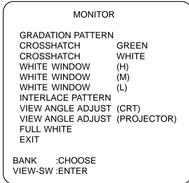
3. Lean the bike to select a test and press 'View Change' to enter the test and to return to "Monitor Menu" from a test.
