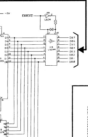
The High Score Memory circuit consists of an erasable reprogrammable ROM N9, latches L9, P9, N10 buffer M9, and timer N11.
