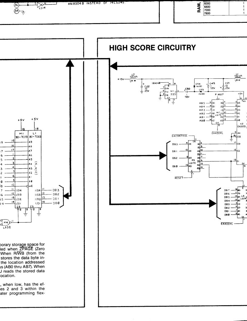
Either a 74LS245 or an AM8304B may be used at location E2. Pin numbers not enclosed in parentheses are for 74LS245. Pin numbers in parentheses are for an AM8304B.
