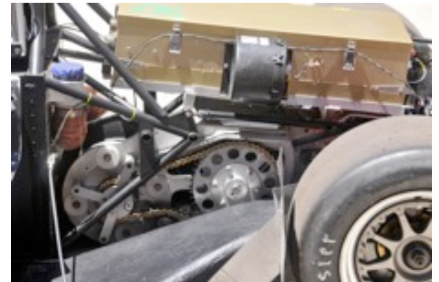
Electro-punk? Closeup of the drive chain on the Kleenspeed electric car
