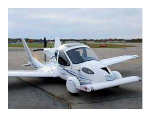
Called the Terrafugia *Transition* it can transform from a two-seater car to a plane in 15 seconds. The manufacturer claims it's easy to keep and run since it uses normal unleaded fuel and fits into a garage. The head of Terrafugia, said: "This is the first really integrated design where the wings fold up automatically and all the parts are in one vehicle."
