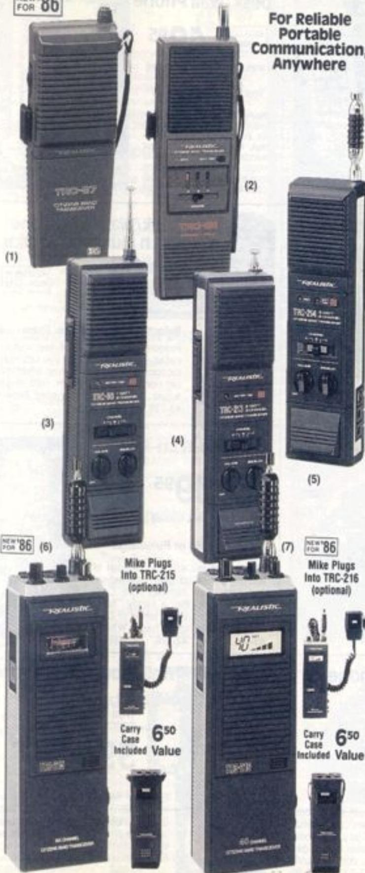
(1) **Realistic TRC-87. 1 Channel, 100 mW.** Sensitive superhet receiver, up-front speaker/mike, side-mounted volume/on-off control and push-to-talk button. Telescoping antenna. With channel 14 crystals, wrist strap.  $6\frac{3}{8} \times 3 \times 1\frac{3}{4}$ ". Requires 9V cell. 21-1609 ..... 19.95
