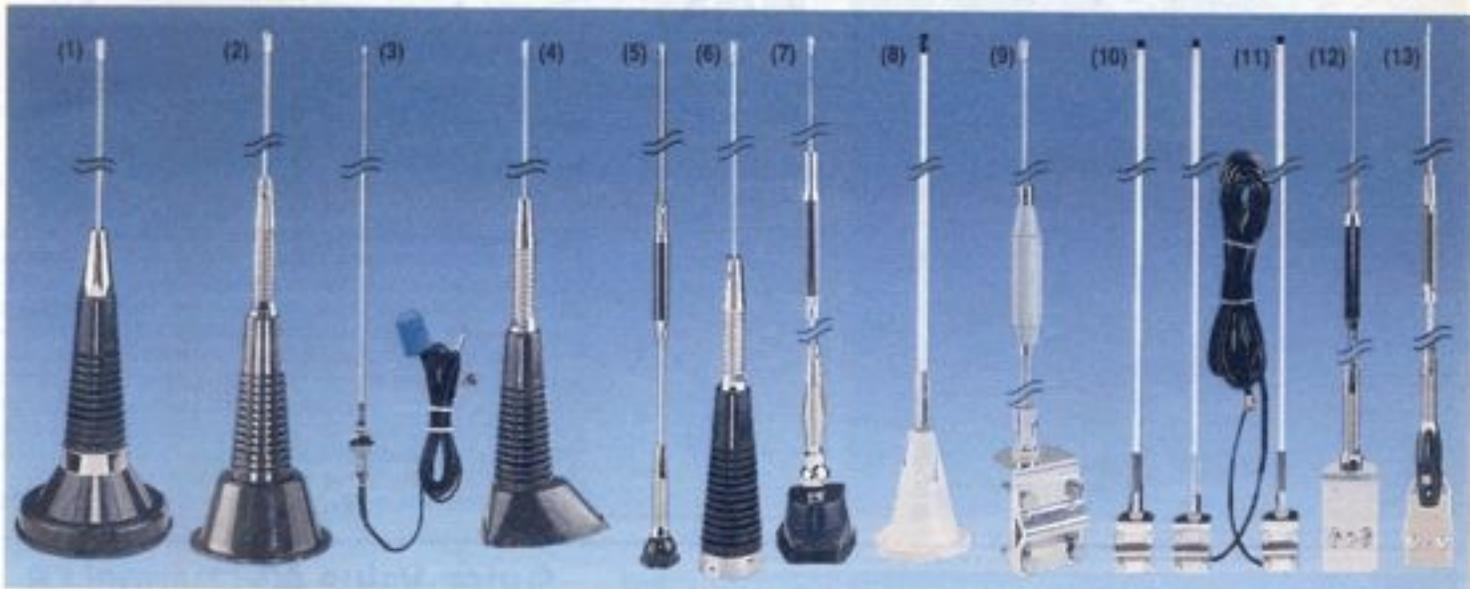
(1) **Deluxe Magnet-Mount.** No holes to drill. It mounts on any flat magnet-holding surface and remains in place at highway speeds. Low-loss coil form, 54" whip. Includes 16-foot cable and PL-259 connector. 21-960 ..... 37.95
