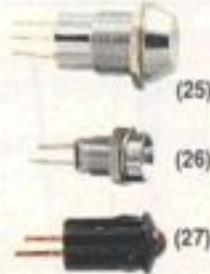
(25) **Two-Color.** 3-lead, 2-segment device provides red and green output. A good mode or status indicator. Requires 3 VDC at 10 mA per segment. Mounts in 3/16" diameter hole. 276-025 ..... 1.49
