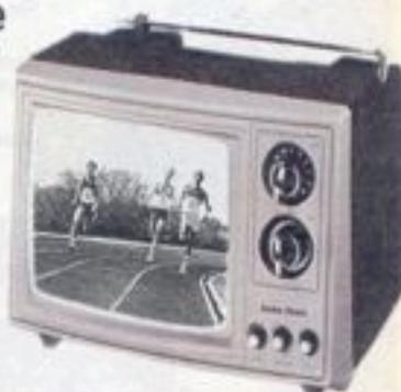
Our lowest priced TV is excellent for kitchen or bedroom. The built-in DC power supply also makes it perfect for vans and camping. Rotary tuning with UHF channel detents. Rugged molded case with handle. Telescoping antenna, terminals for external 75/300-ohm antenna. With earphone. 8<sup>7</sup>/<sub>8</sub> x 10<sup>1</sup>/<sub>4</sub> x 12<sup>1</sup>/<sub>8</sub>". UL listed AC or 12VDC neg. gnd. 16-240 ..... 99.95
