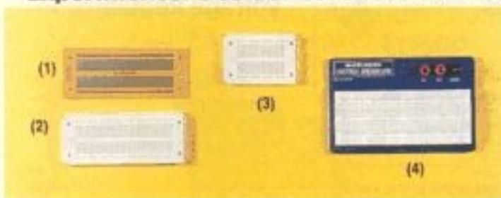
The fast and efficient way to design your own circuits. The modular breadboards are reusable and accept a wide variety of components. When you have your circuit working properly, it's easy to transfer it from the breadboard to the matching experimenter's PC board for a soldered, permanent version.
