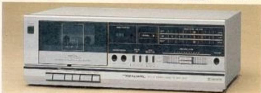
**Response**  $\pm 3$  dB: 40-14,000 Hz (metal), 40-13,000 Hz (CrO<sub>2</sub>/Hi-Bias), 40-12,000 Hz (normal). **Wow and Flutter:** 0.17% WRMS. **S/N:** 67 dB Dolby C (ref. 3.0% distortion, "A" weighted, metal tape). **Distortion:** 1.5% 3rd HD. **Record/Play Head:** Permalloy. **Erase Head:** Ferrite. **Size:** 4 $\frac{1}{16}$ " x 15 $\frac{1}{16}$ " x 9 $\frac{1}{4}$ ". \*TM Dolby Laboratories Licensing Corp.
