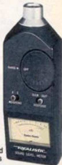
Great for adjusting equalizers, PA systems or checking sound levels in schools, offices, factories. Reads to 126 dB SPL with slow and fast response settings. "A" or "C" weighting. Electret mike, tape recording output, socket for mounting on tripod. 6 1/4 x 2 7/16 x 1 3/4". Requires 9V cell. 33-2050 ..... 29.95
