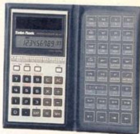
Radio Shack EC-4013. Separate keyboards for binary, octal, and hexadecimal calculations/conversions, as well as logical operations. With 13 special physical constants and 16 metric conversion functions. Has a 10-digit mantissa and 2-digit exponent. 5 x 3 1/4 x 9/16". 65-930 ..... 34.95
